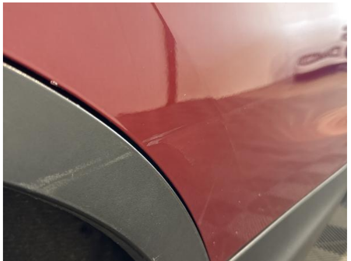
12: Door osr Dented With Paint Damage
