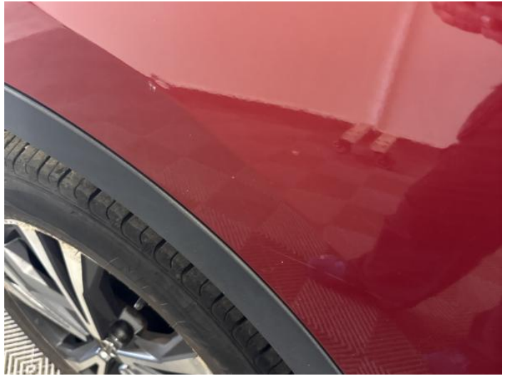
4: Wing nsf Scratched Over 25mm Thru Paint
