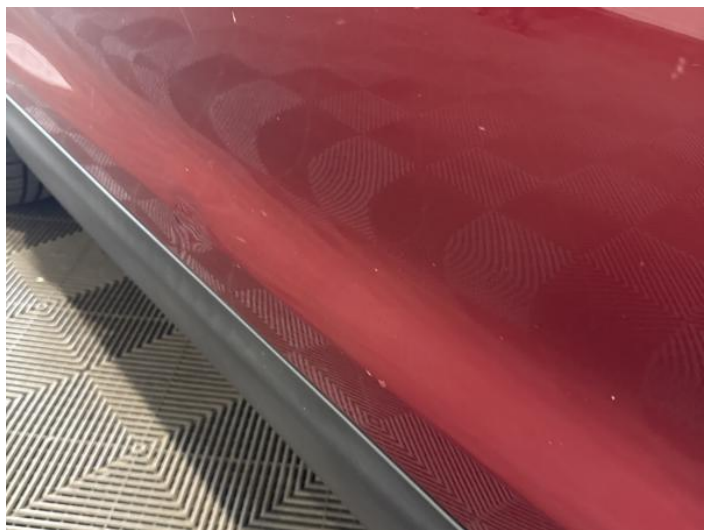
8: Door nsf Dented Over 30mm
