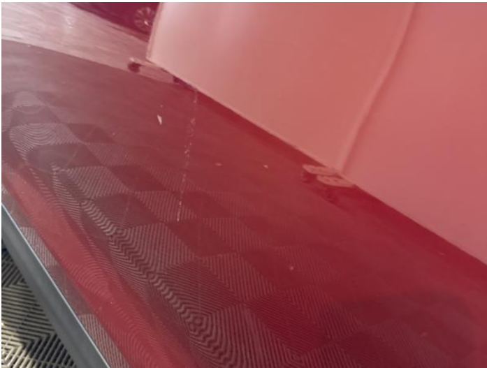
5: Door nsf Scratched Over 25mm Thru Paint
