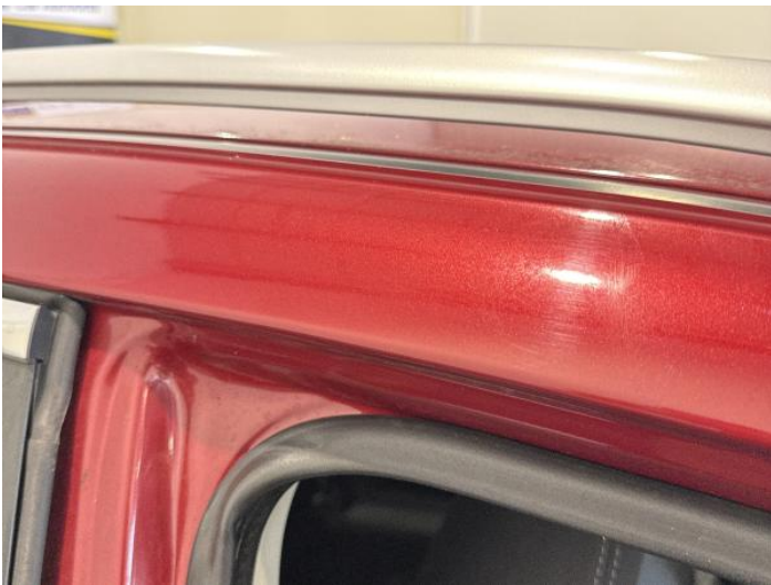
17: A Post of Poor Previous Repair Poor Paint
