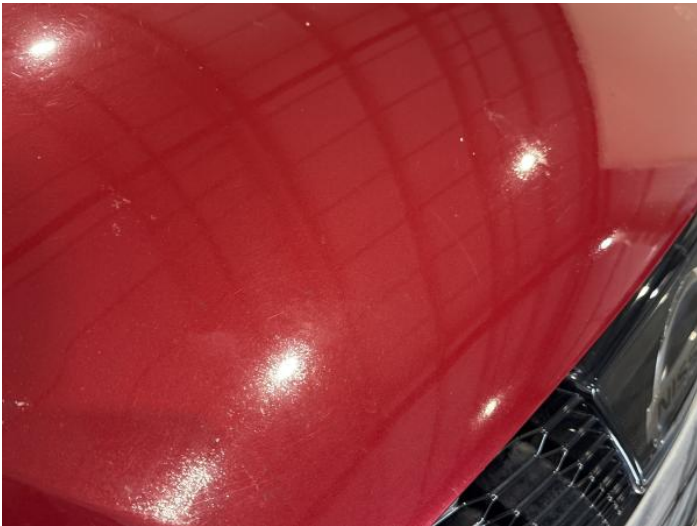
1: Bonnet Poor Previous Repair Poor Paint
