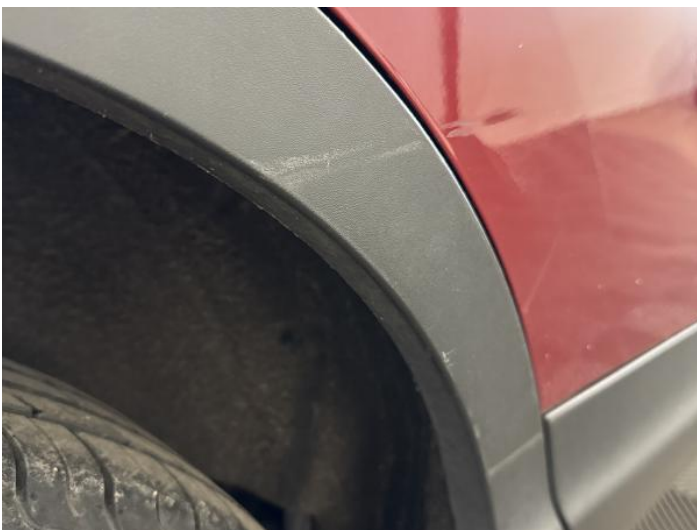
13: Qtr Panel Arch Extension os Scuffed (Unpainted) Over 100mm
