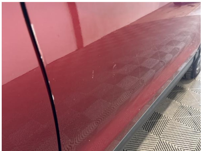
14: Door osf Scratched Over 25mm Thru Paint
