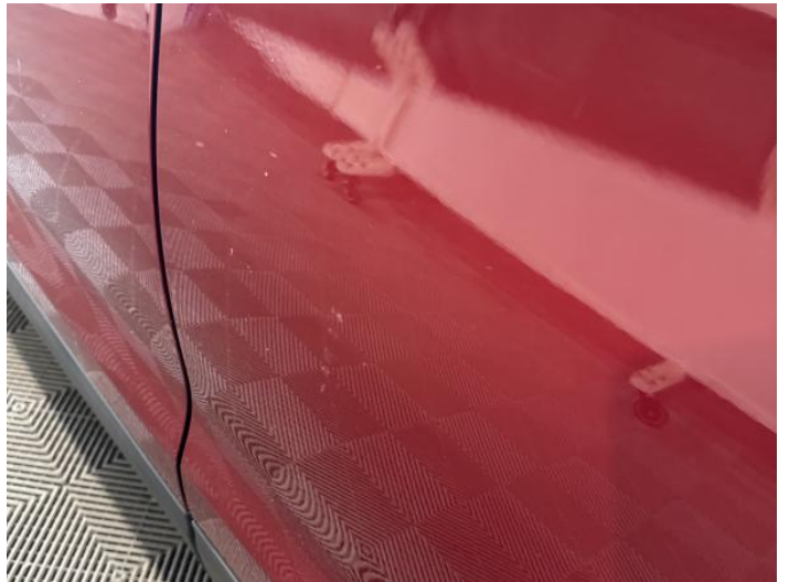
6: Door nsr Scratched Over 25mm Thru Paint
