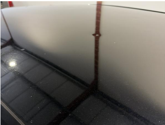
11: Roof Dented Over 30mm
