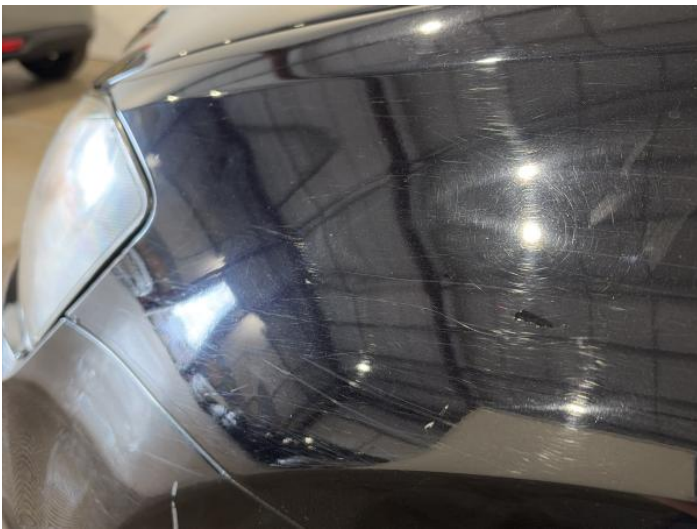
5: Wing nsf Scratched Over 25mm Thru Paint
