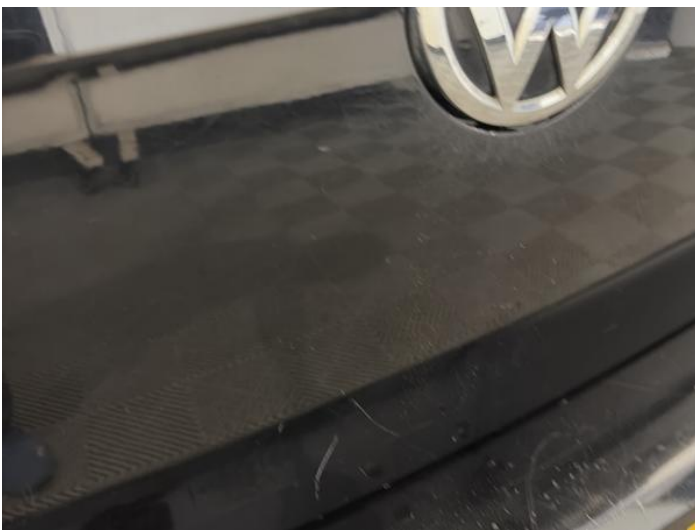
13: Tailgate Scratched Over 25mm Thru Paint
