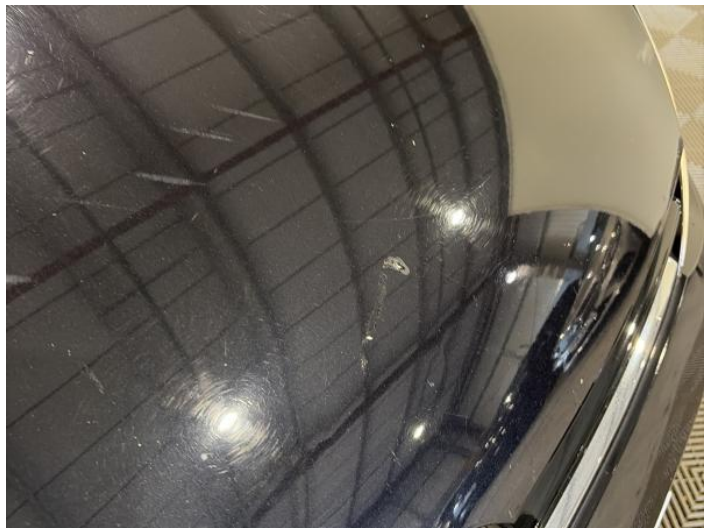
2: Bonnet Scratched Over 25mm Thru Paint
