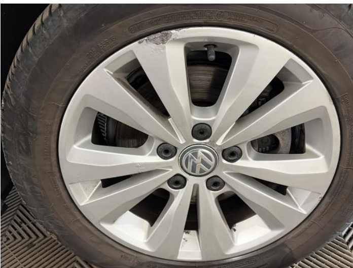
19: Wheel osf Scratched Over 50mm
