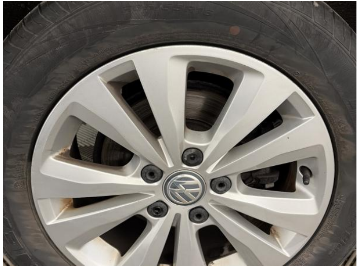
16: Wheel osr Scratched Up To 50mm
