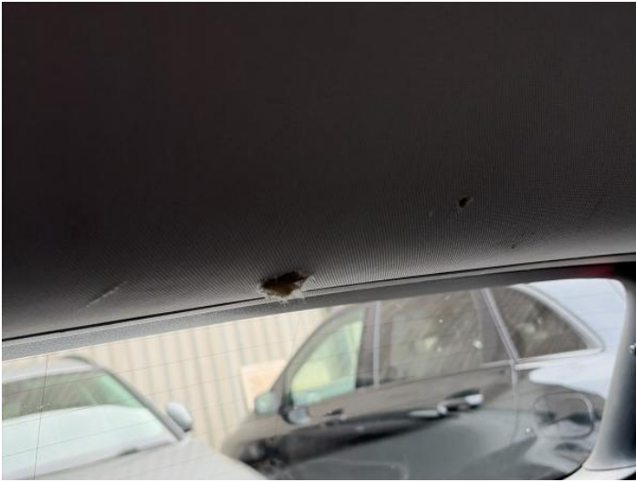
21: Roof Lining Torn Over 3mm
