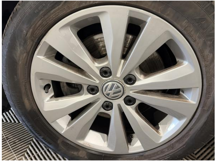
4: Wheel nsf Scratched Up To 50mm
