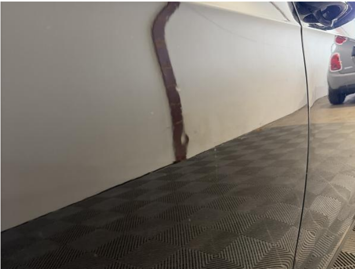
17: Door osr Dented Between 10mm + 30mm
