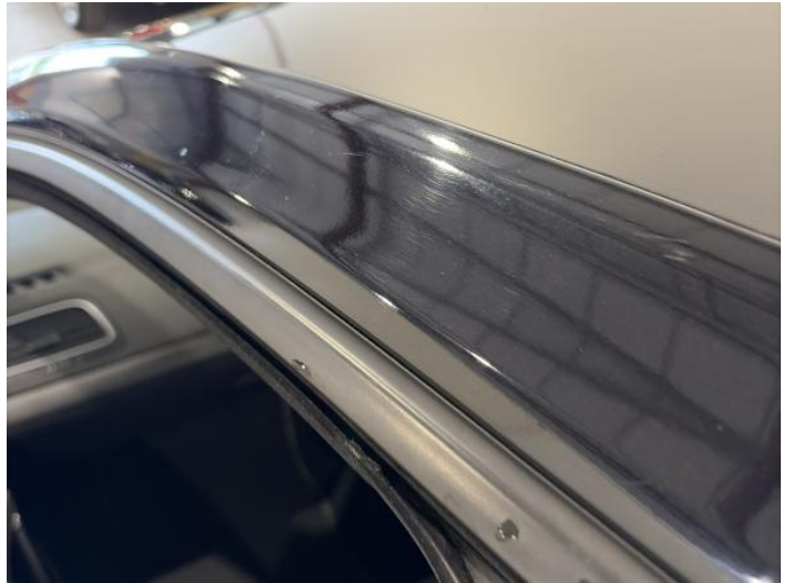
10: A Post ns Dented Between 10mm + 30mm
