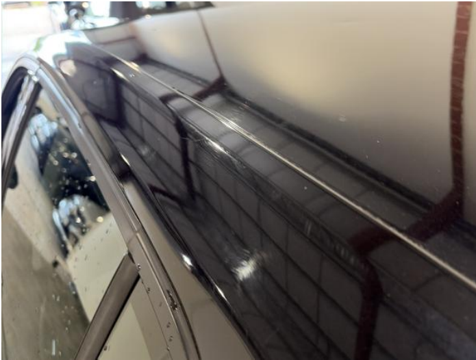
9: B Post ns Dented Between 10mm + 30mm
