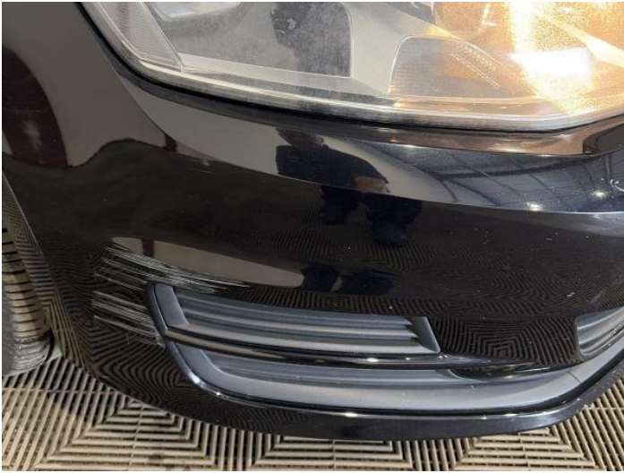
3: Bumper Front Scratched Over 100mm Thru Paint
