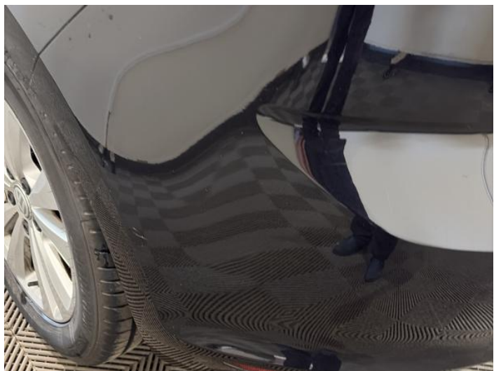
14: Bumper Rear Scratched Over 100mm Thru Paint
