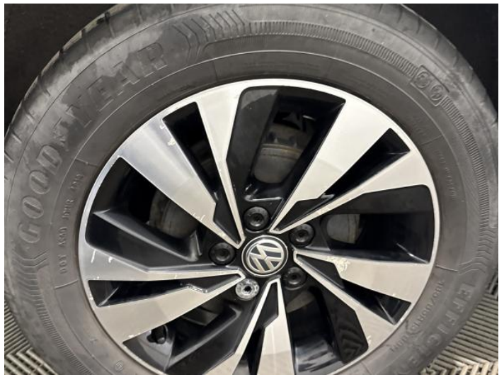
12: Wheel osr Scratched Over 50mm
