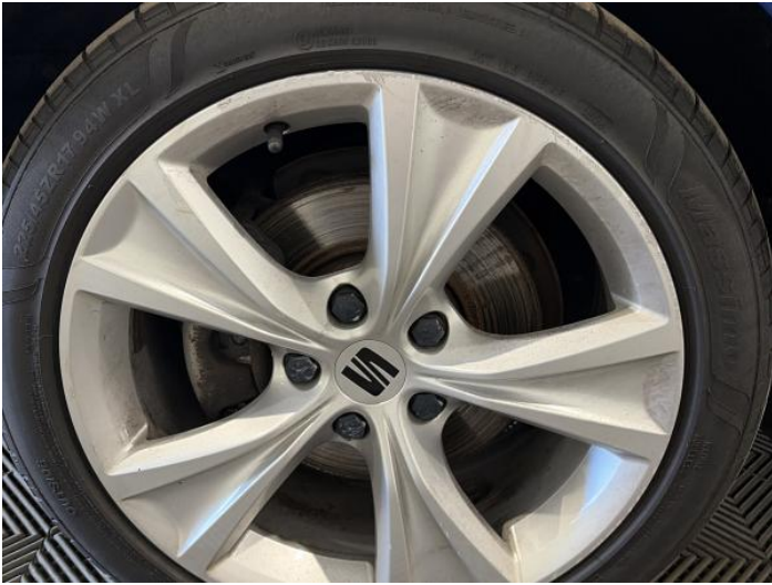
3: Wheel nsf Scratched Over 50mm
