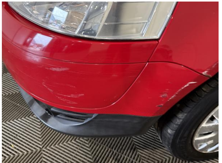
2: Bumper Front Scratched Over 100mm Thru Paint
