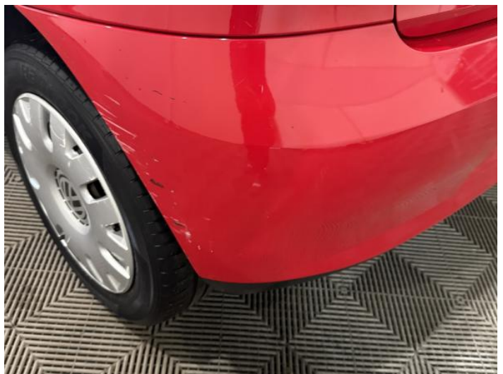
8: Bumper Rear Scratched Over 100mm Thru Paint
