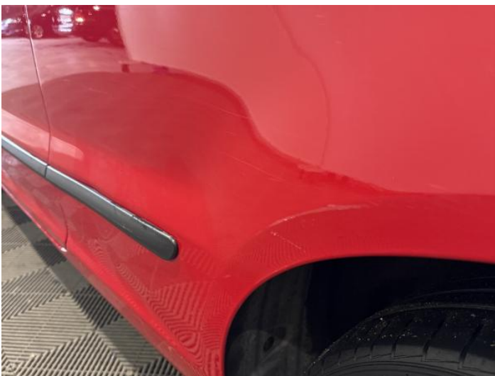
7: Qtr Panel nsr Dented With Paint Damage
