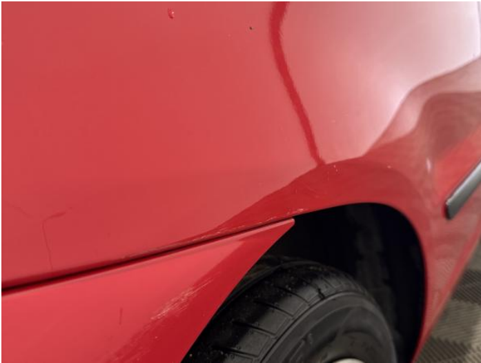
9: Qtr Panel osr Scratched Over 25mm Thru Paint
