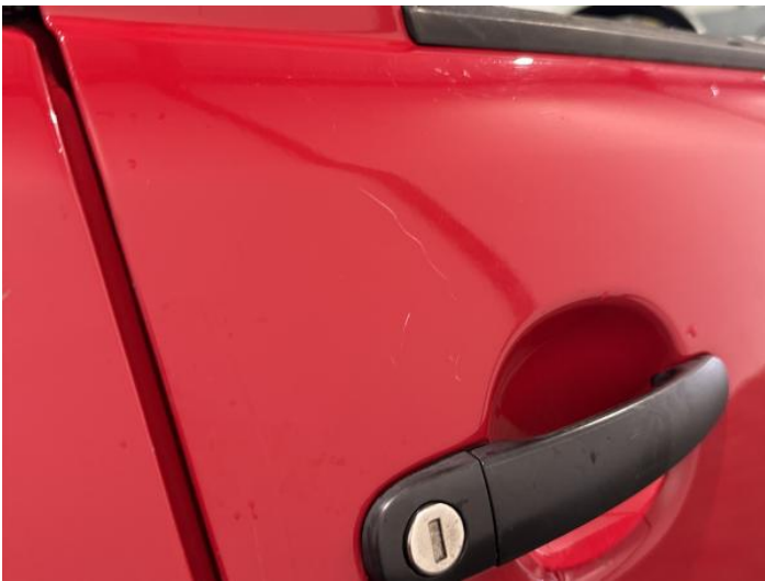
11: Door osf Scratched Over 25mm Thru Paint
