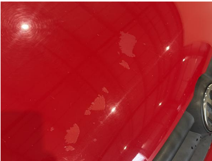
1: Bonnet Poor Previous Repair Paint Flake
