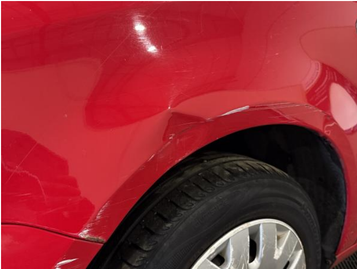
3: Wing nsf Dented With Paint Damage
