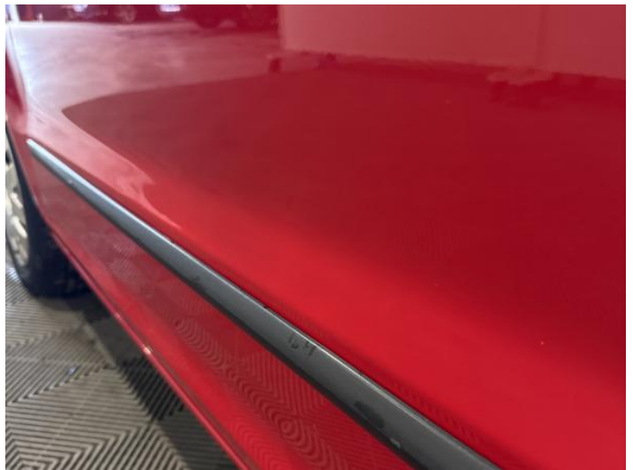
6: Door nsf Dented Over 30mm
