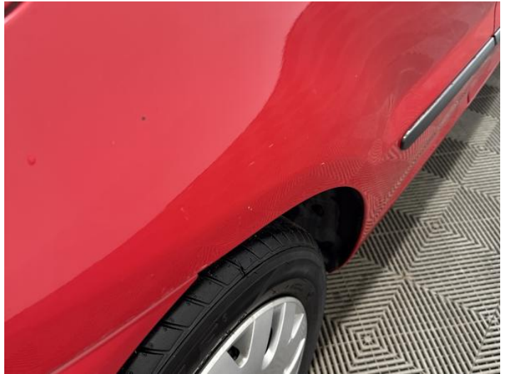
10: Qtr Panel osr Dented Between 10mm + 30mm
