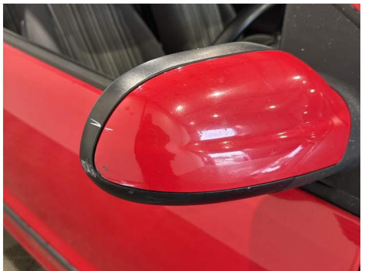
14: Door Mirror Assy osf Scratched (Painted) UpTo 25mm Thru Paint
