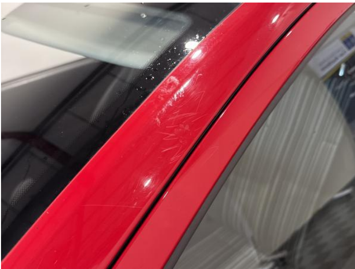
5: A Post ns Scratched Over 25mm Thru Paint
