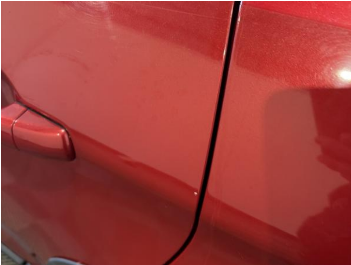
9: Door nsr Poor Previous Repair Poor Paint
