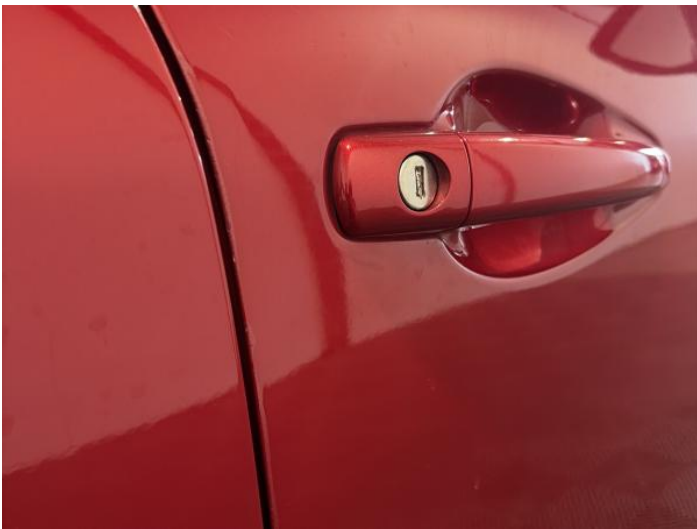
11: Door osf Chipped Edge Chip
