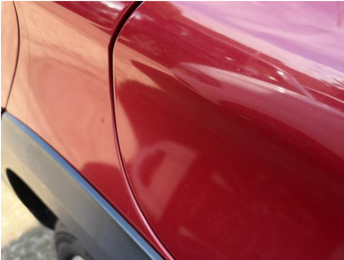
15: Qtr Panel nsr Poor Previous Repair Poor Paint
