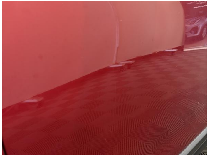
6: Door nsf Poor Previous Repair Poor Paint
