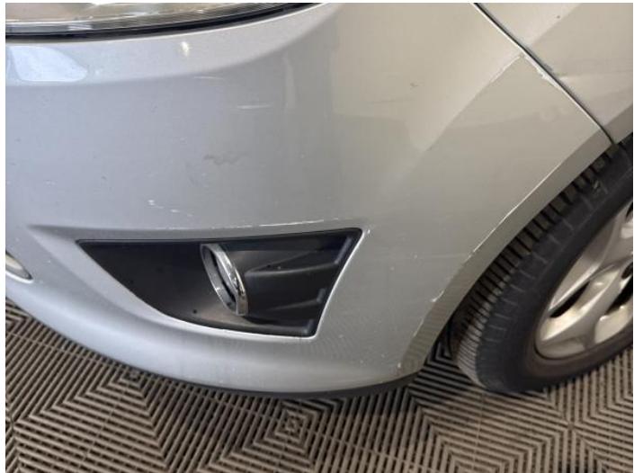
2: Bumper Front Scratched Over 100mm Thru Paint
