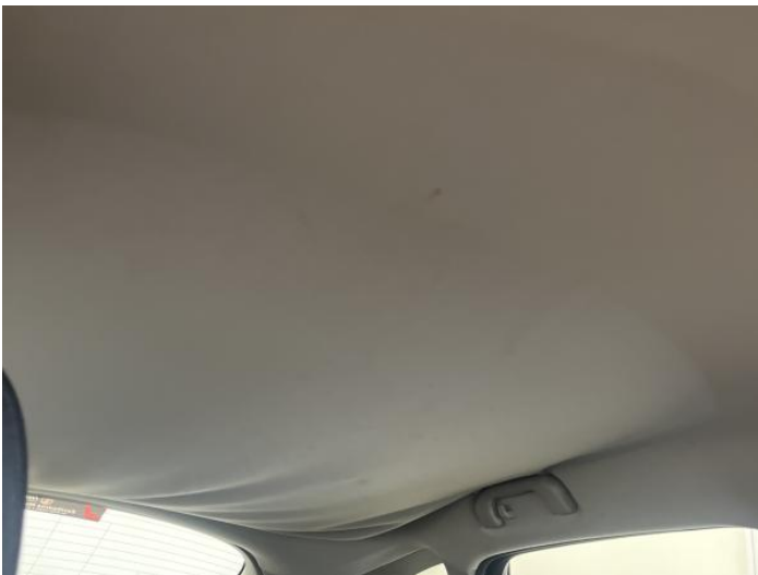
1: Roof Lining Scuffed Over 25mm
