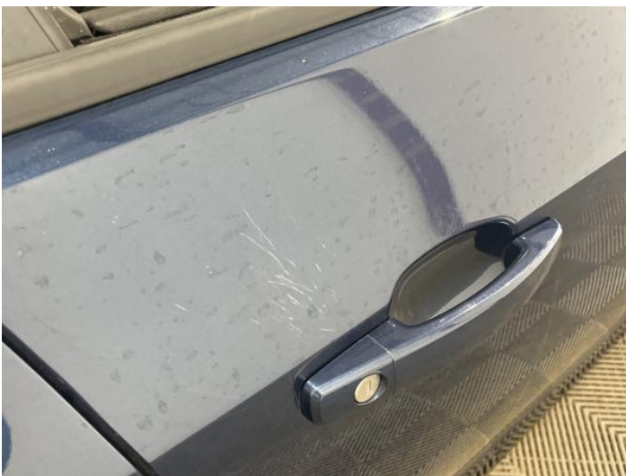
13: Door osf Scratched Over 25mm Thru Paint
