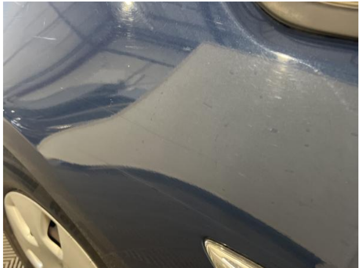
6: Wing nsf Scratched Over 25mm Thru Paint
