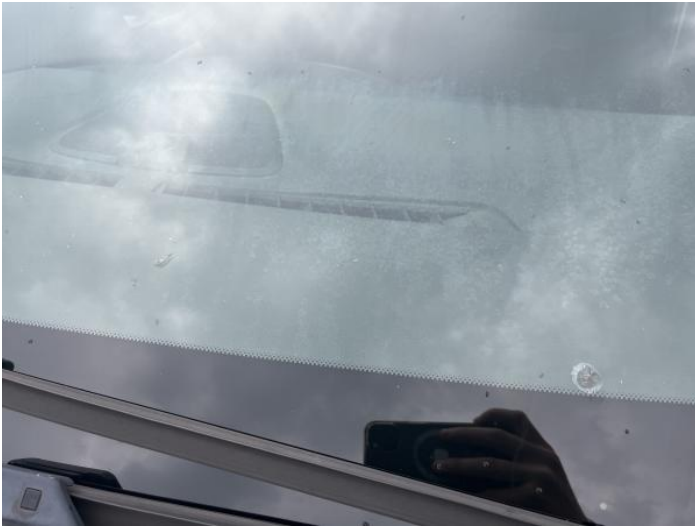
15: Screen Front Chipped Over 10mm
