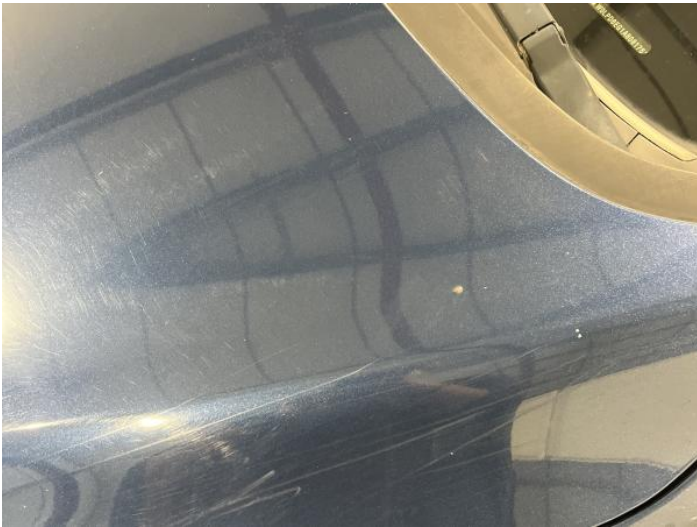
5: Bonnet Scratched Over 25mm Thru Paint
