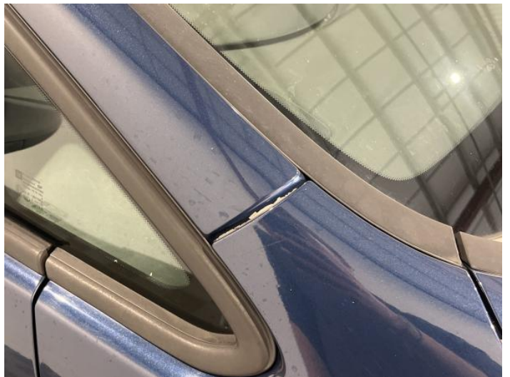
2: A Post os Poor Previous Repair Paint Flake
