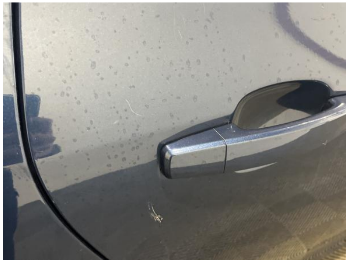
12: Door osr Scratched Over 25mm Thru Paint
