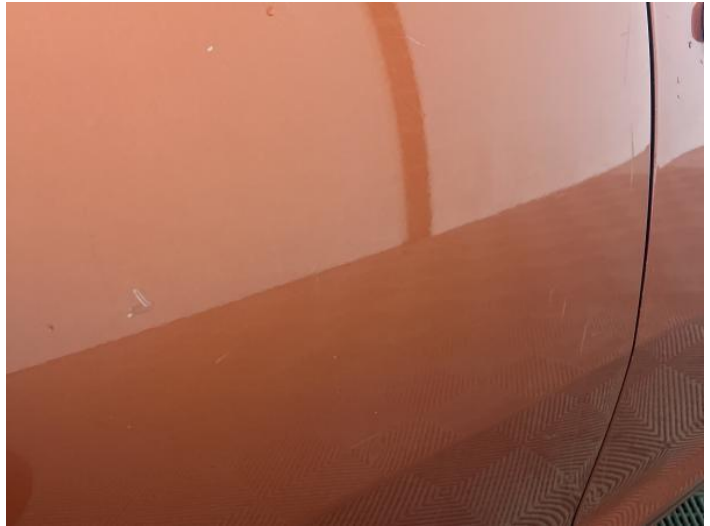
10: Door osr Scratched Over 25mm Thru Paint
