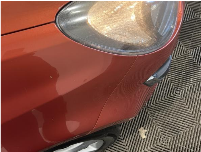
1: Wing of Poor Previous Repair Poor Colour
