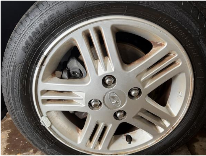
3: Wheel nsf Scratched Over 50mm
