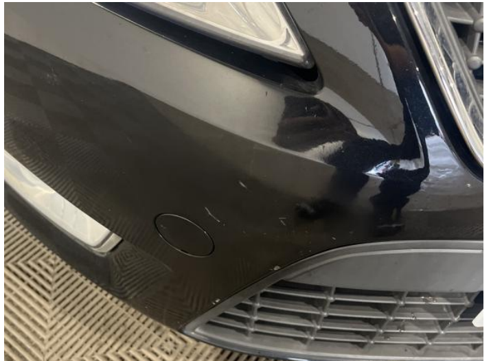
2: Bumper Front Scratched 25 to 100mm Thru Paint
