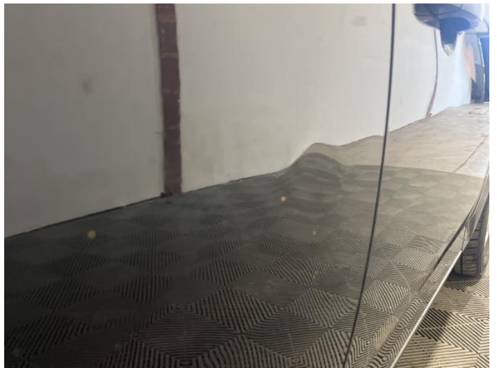
12: Door osr Dented Over 30mm
