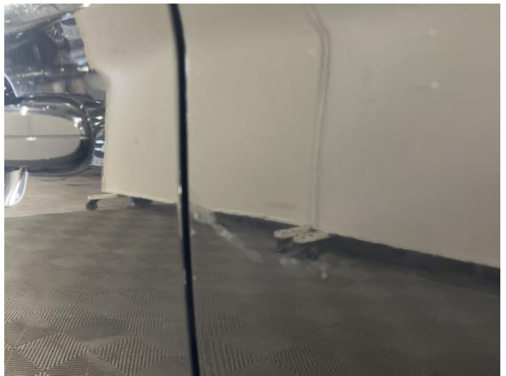
6: Door nsr Scratched Over 25mm Thru Paint
