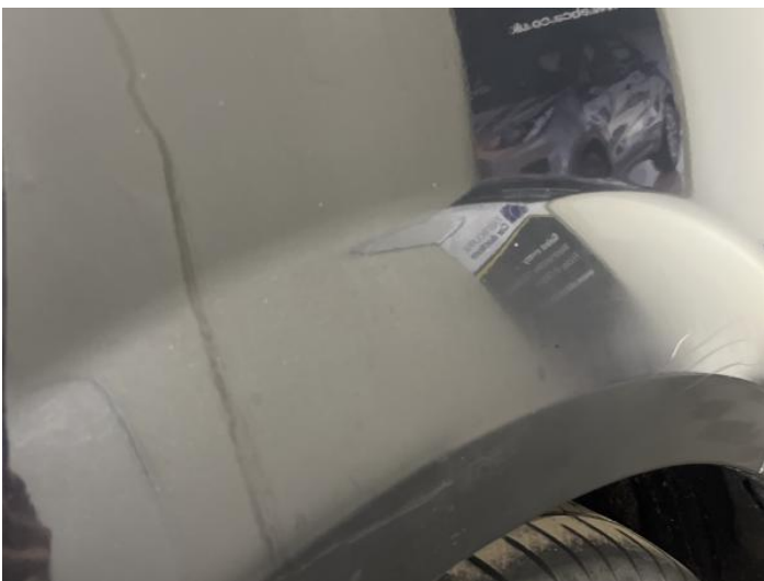
7: Qtr Panel nsr Poor Previous Repair Poor Paint
