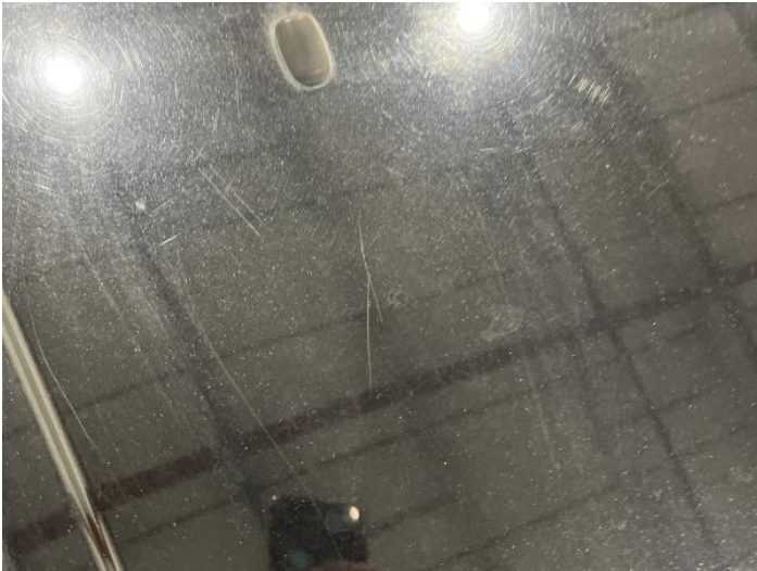
3: Bonnet Scratched Over 25mm Thru Paint
