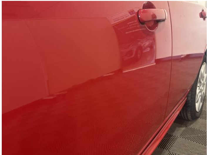
6: Door nsf Dented With Paint Damage
