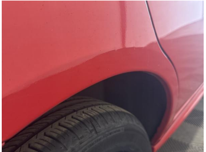
10: Qtr Panel osr Dented Over 30mm
