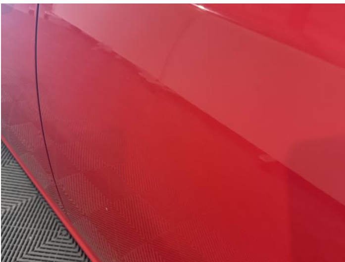
7: Door nsr Dented With Paint Damage
