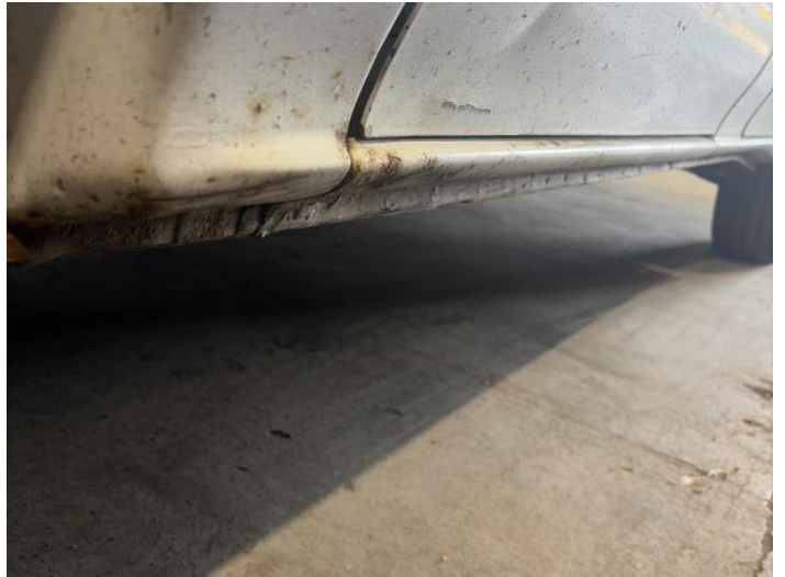
4: Sill os Rusted Over 5mm
