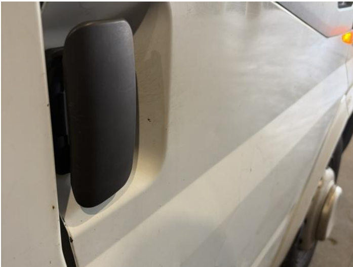
5: Door osf Dented With Paint Damage
