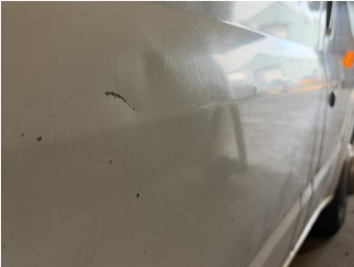
3: Door osr Dented With Paint Damage
