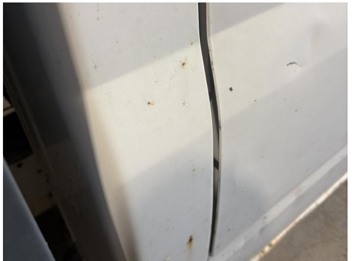
2: B Post os Rusted Over 5mm
