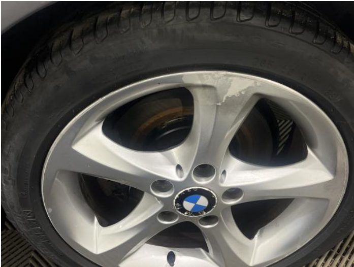
9: Wheel nsr Scratched Over 50mm
