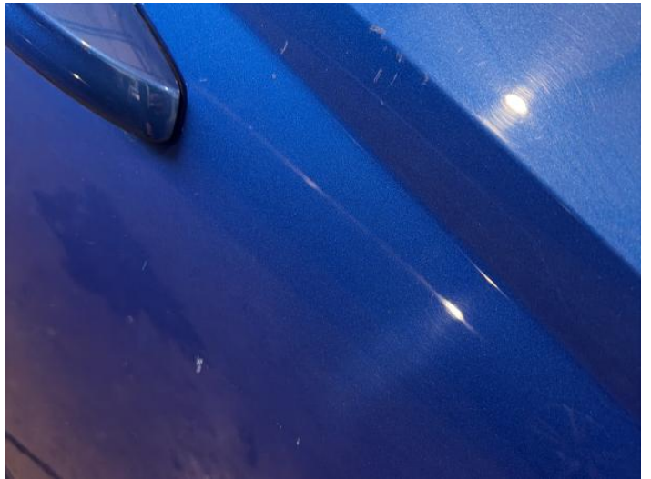
6: Door osf Chipped Multiple Chips
