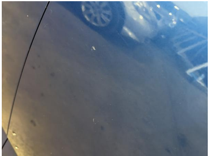
14: Door nsr Chipped 1 To 5
