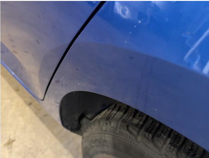
11: Qtr Panel nsr Dented Between 10mm + 30mm
