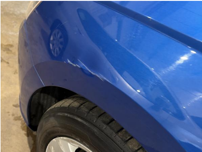
17: Wing nsf Dented With Paint Damage
