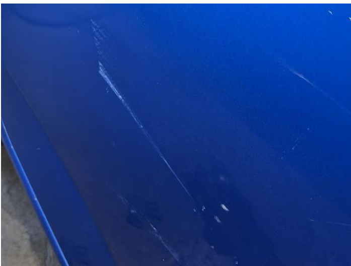
7: Door osr Scratched Over 25mm Thru Paint
