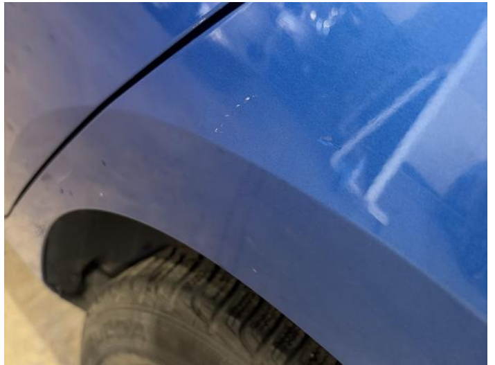
12: Qtr Panel nsr Chipped 1 To 5
