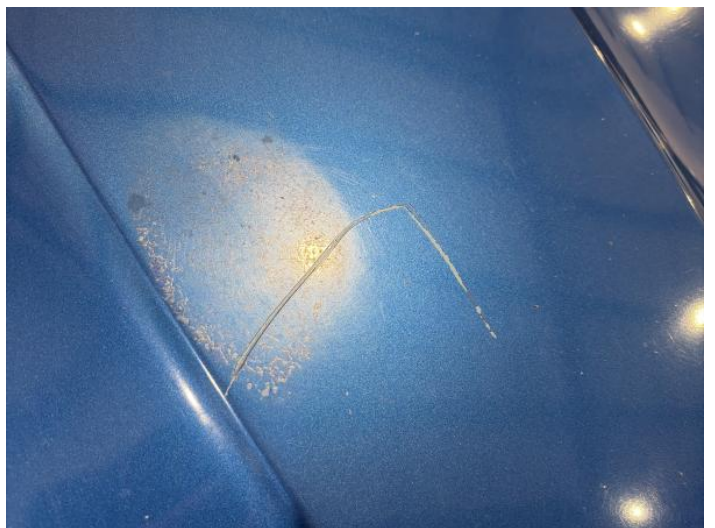
20: Bonnet Scratched Over 25mm Thru Paint
