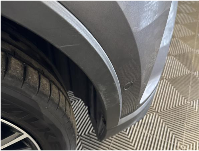
15: Wing Front Arch Extension os Scuffed (Unpainted) Over 100mm
