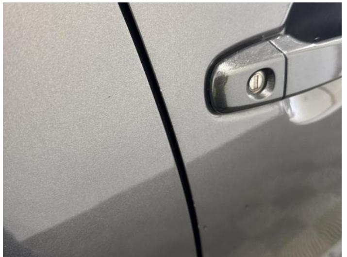
12: Door osr Scratched UpTo 25mm Thru Paint
