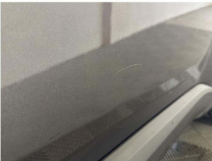
13: Door osf Scratched Over 25mm Thru Paint
