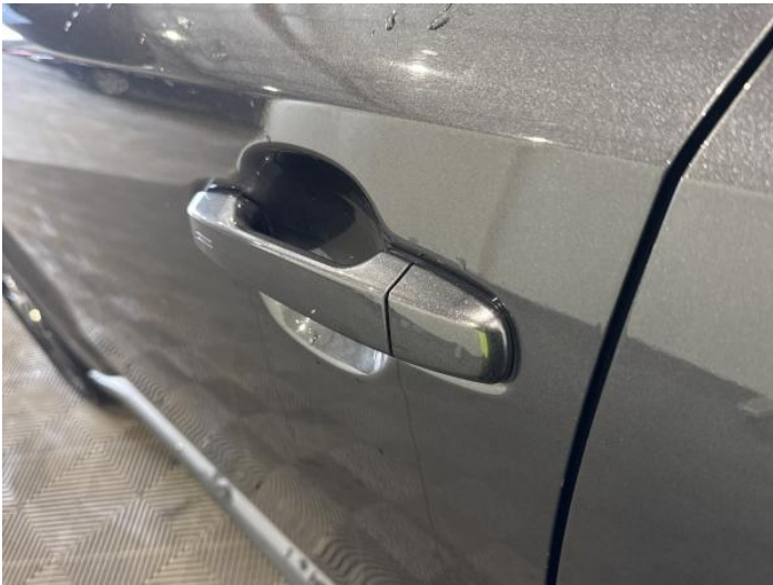
5: Door nsf Dented With Paint Damage
