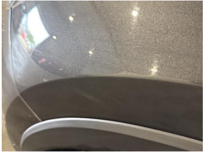
4: Wing nsf Scratched Over 25mm Thru Paint
