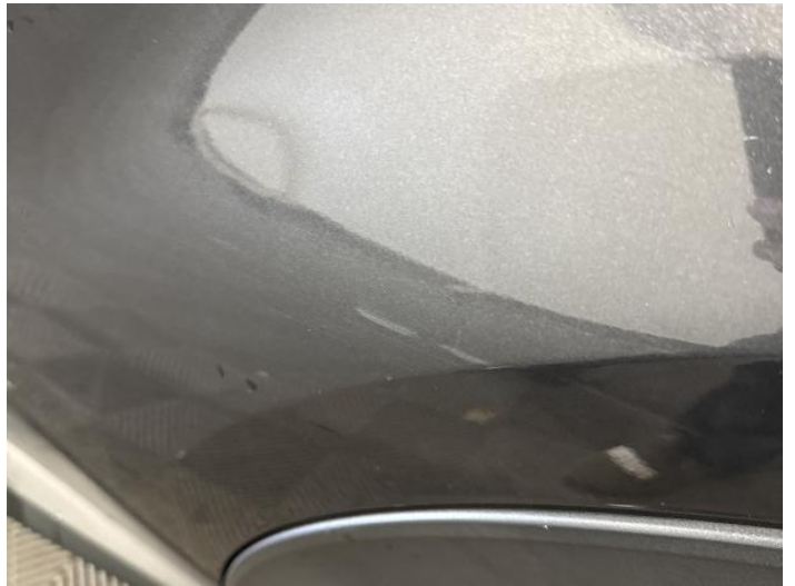
6: Door nsr Scratched Over 25mm Thru Paint
