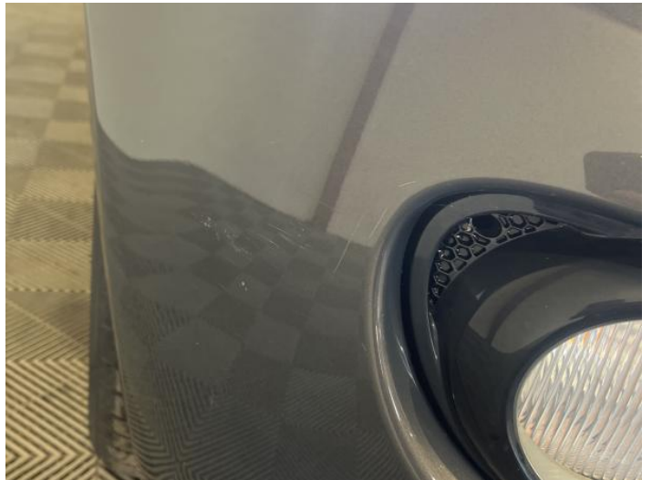
2: Bumper Front Scratched 25 to 100mm Thru Paint
