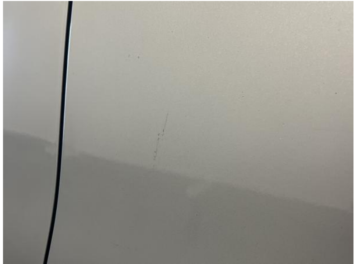
10: Door nsr Scratched Over 25mm Thru Paint
