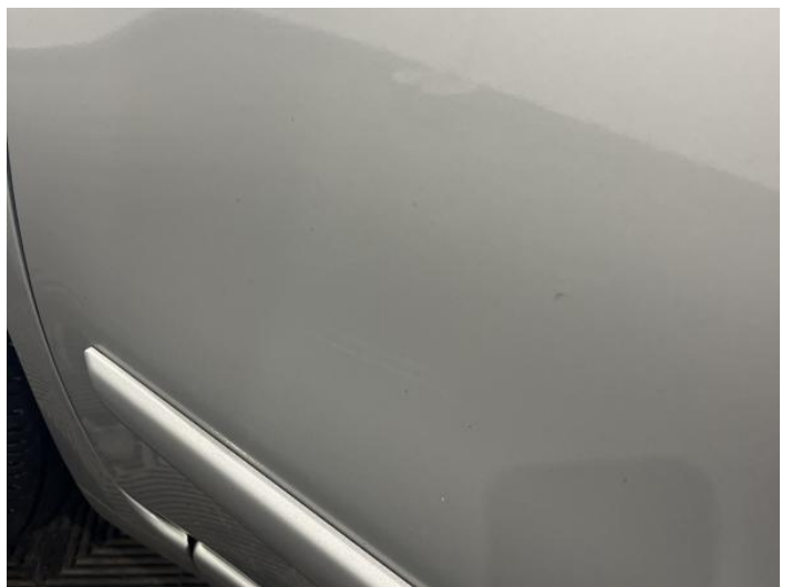
8: Door nsf Scratched Over 25mm Thru Paint
