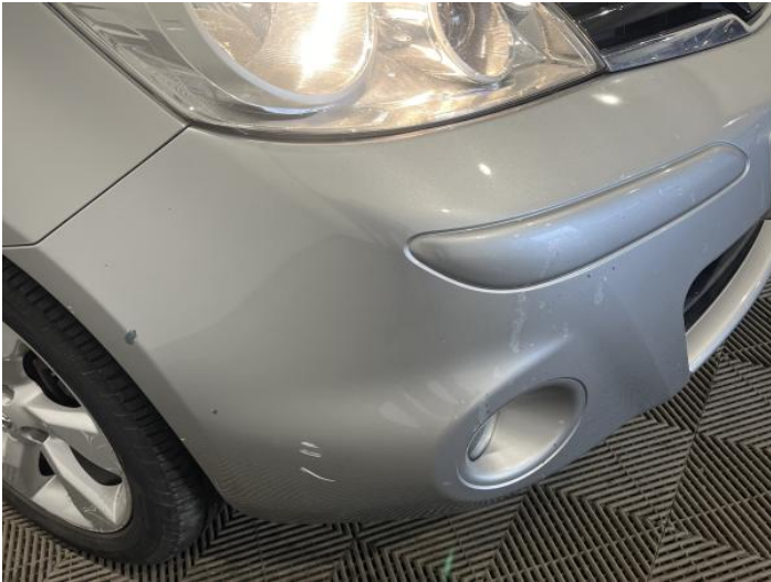
3: Bumper Front Scratched Over 100mm Thru Paint
