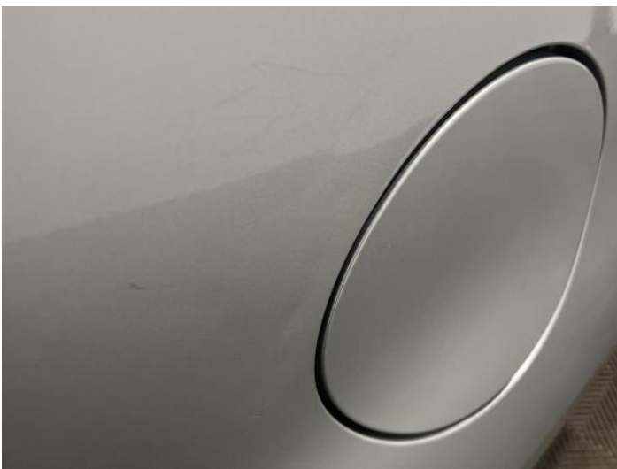
13: Qtr Panel osr Poor Previous Repair Rippled UpTo 30%
