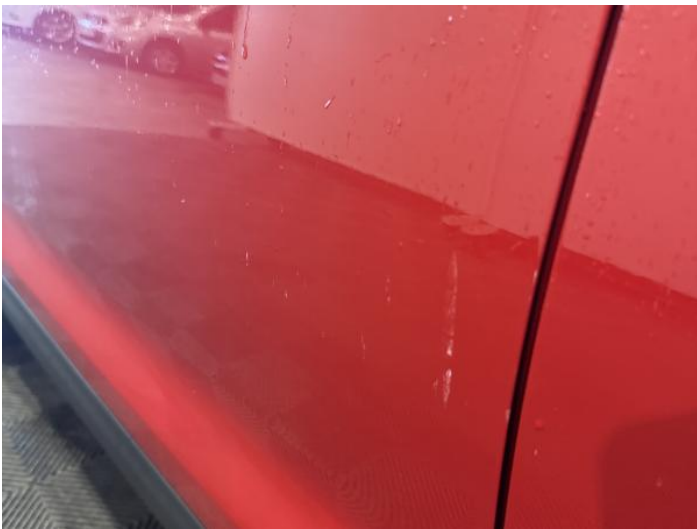
5: Door nsf Scratched Over 25mm Thru Paint
