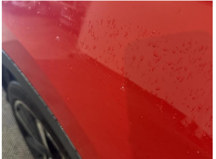
4: Wing nsf Scratched Over 25mm Thru Paint
