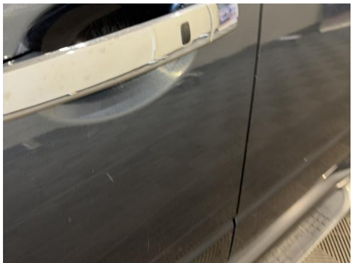
8: Door nsf Dented Between 10mm + 30mm
