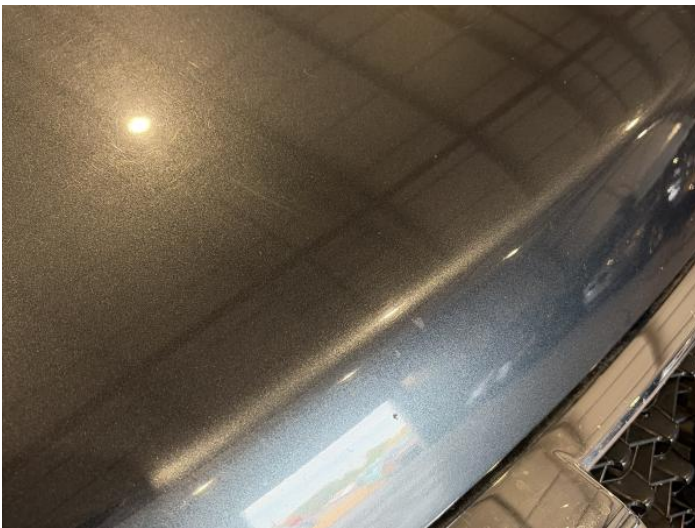
1: Bonnet Scratched Over 25mm Thru Paint
