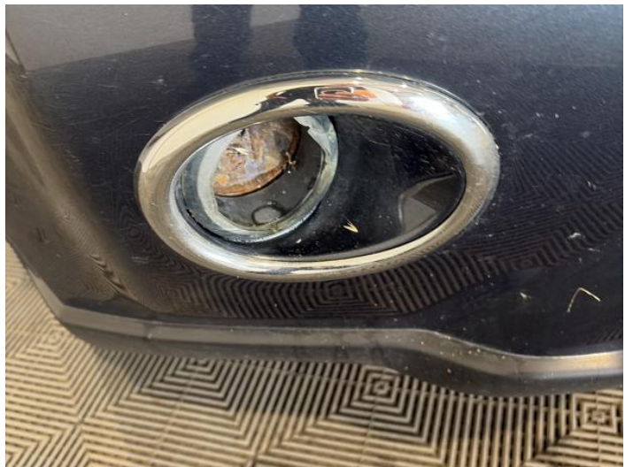
2: Fogdriving Lamp osf Broken Replace
