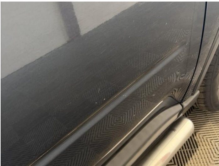
17: Door osf Scratched Over 25mm Thru Paint
