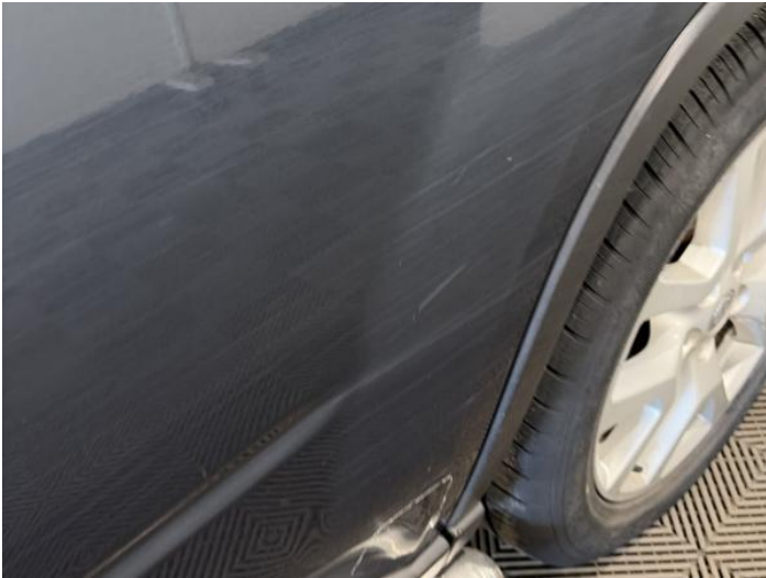
9: Door nsr Scratched Over 25mm Thru Paint
