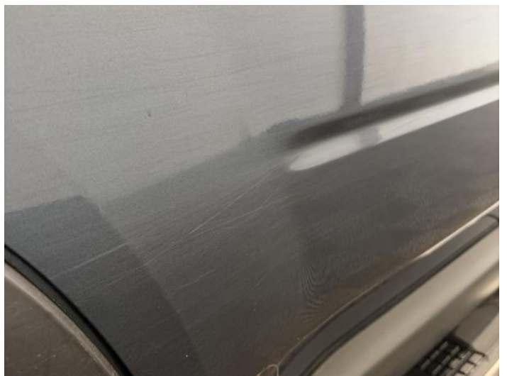
14: Door nsr Scratched Over 25mm Thru Paint
