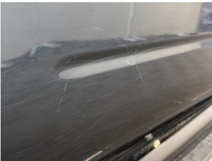
7: Door nsf Scratched Over 25mm Thru Paint
