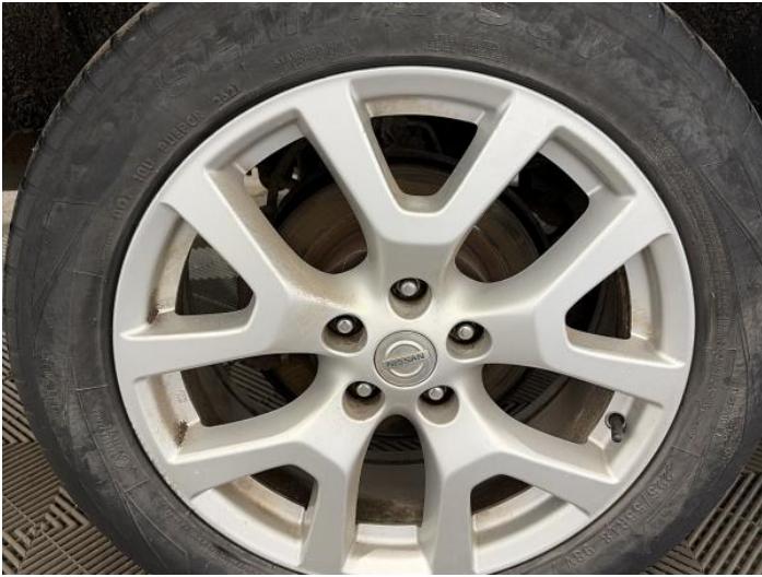
15: Wheel osr Scratched Over 50mm
