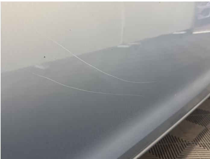
5: Door nsf Scratched Over 25mm Thru Paint
