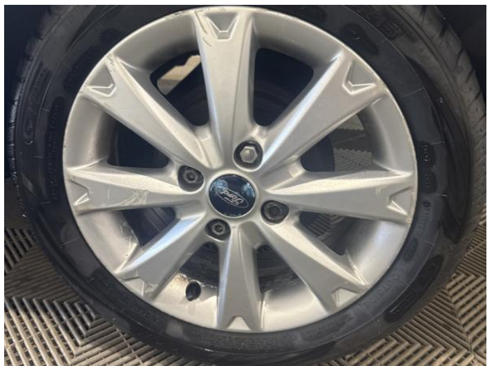
8: Wheel nsr Scratched Over 50mm
