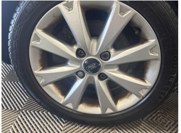
4: Wheel nsf Scratched Over 50mm
