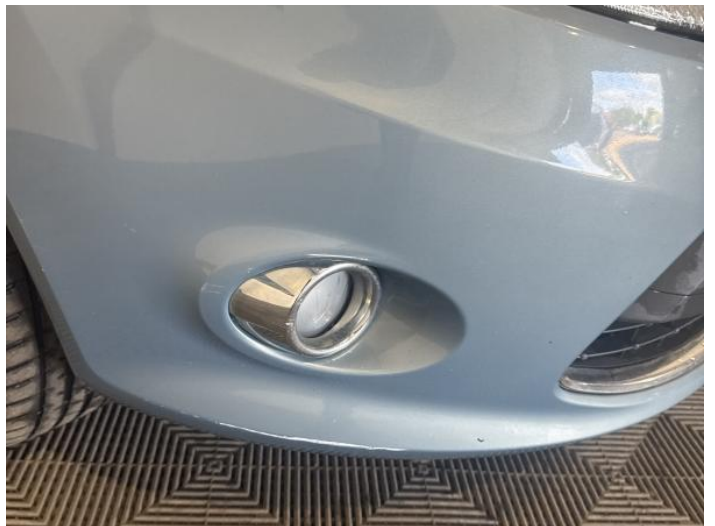
2: Bumper Front Scratched 25 to 100mm Thru Paint
