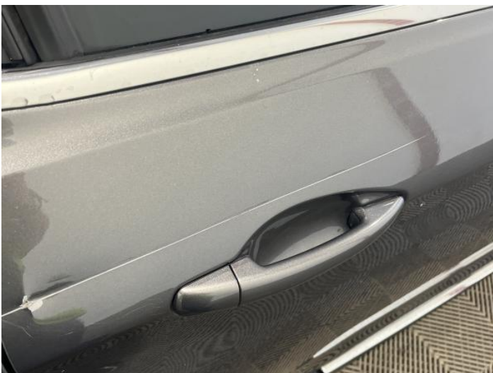
7: Door nsr Dented With Paint Damage
