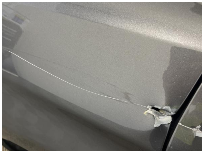
8: Qtr Panel osr Hole Over 10mm
