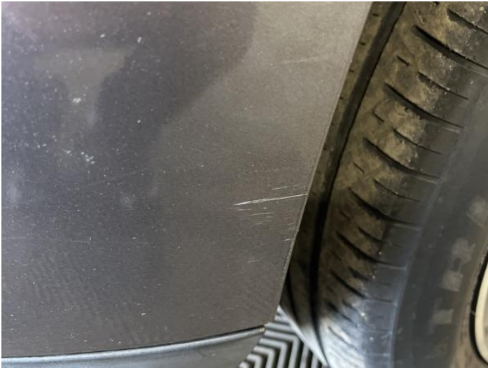
3: Bumper Front Scratched 25 to 100mm Thru Paint
