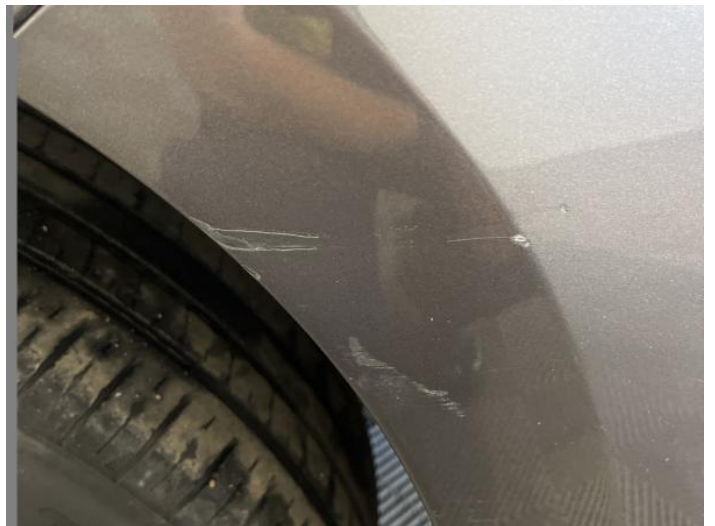
2: Bumper Front Scratched 25 to 100mm Thru Paint
