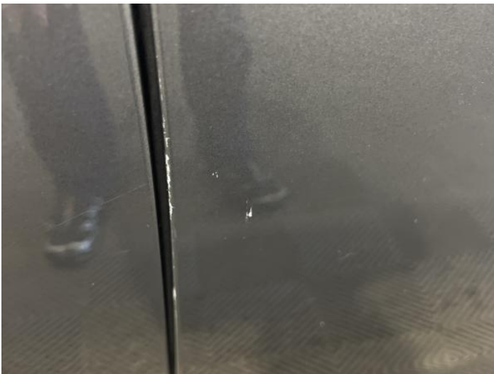
1: Door osf Chipped Multiple Chips
