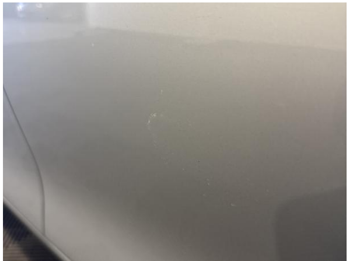
6: Door nsr Scratched Over 25mm Thru Paint
