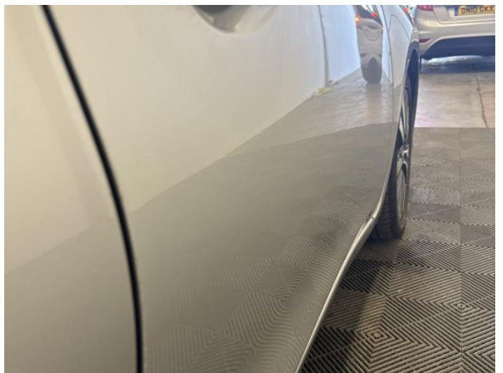
14: Door osf Dented Over 30mm
