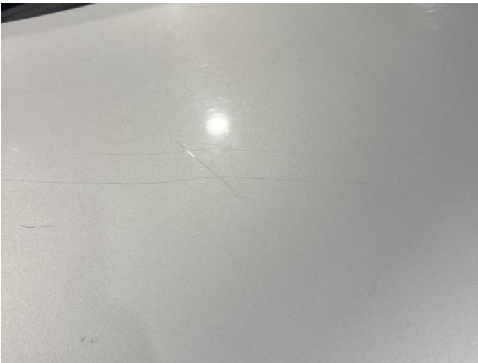
1: Bonnet Scratched Over 25mm Thru Paint
