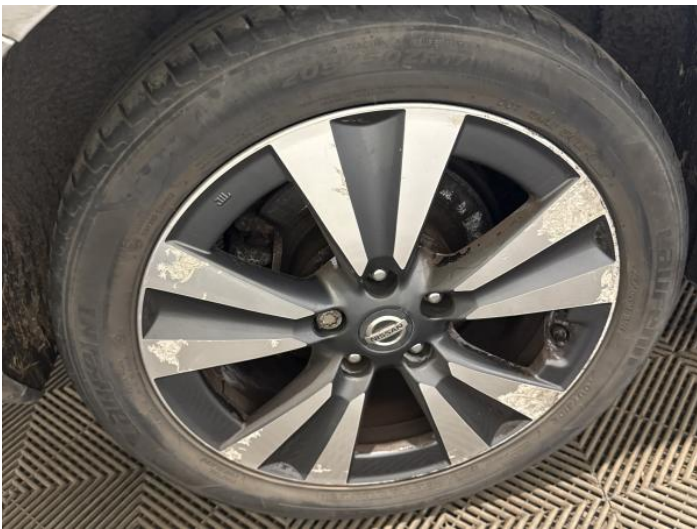
11: Wheel osr Scratched Over 50mm
