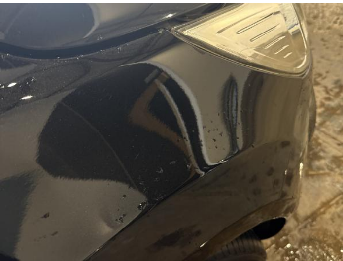
13: Wing osf Poor Previous Repair Poor Paint
