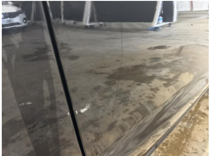
12: Door osf Poor Previous Repair Poor Paint
