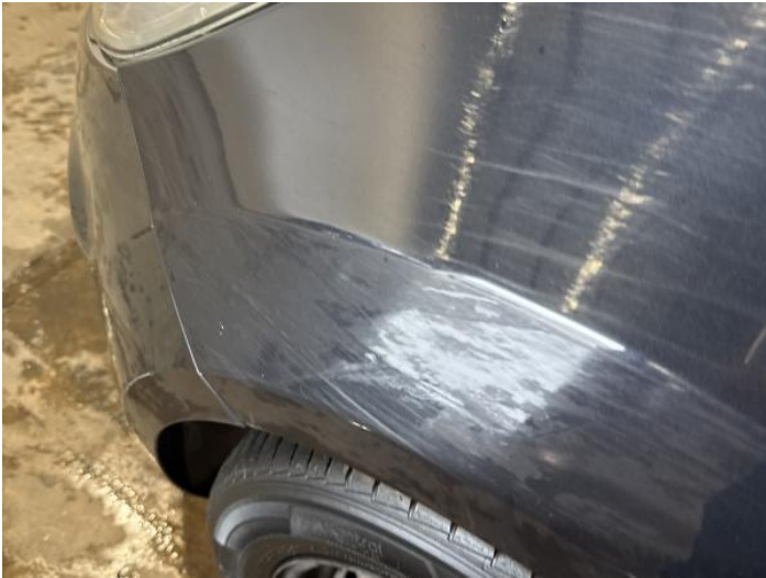
3: Wing nsf Scratched Over 25mm Thru Paint
