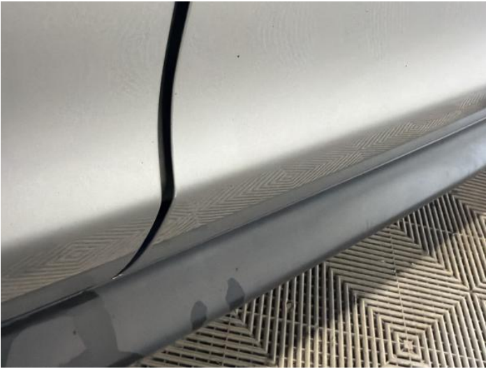
3: Door osf Chipped Edge Chip
