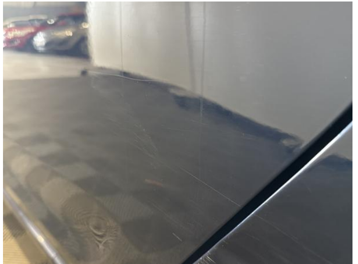
6: Door nsr Scratched Over 25mm Thru Paint
