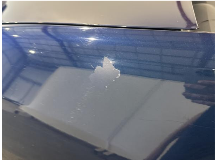
4: Wing nsf Poor Previous Repair Paint Flake
