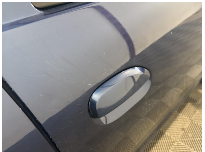
14: Door nsf Dented With Paint Damage
