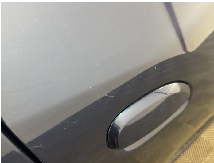
13: Door osr Scratched Over 25mm Thru Paint
