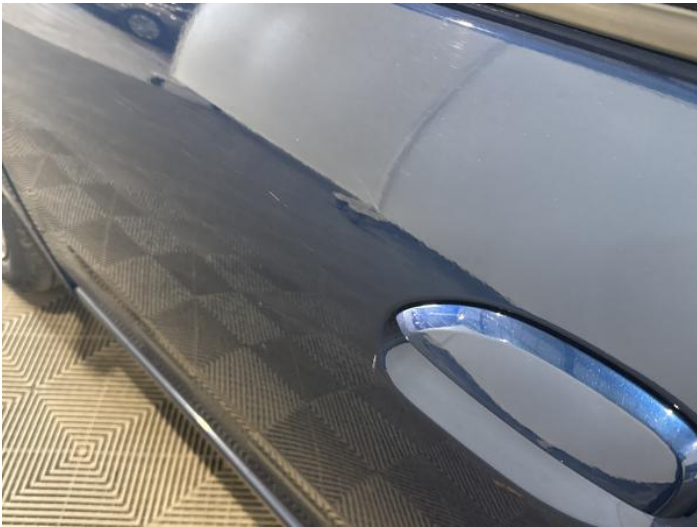
5: Door nsf Scratched Over 25mm Thru Paint
