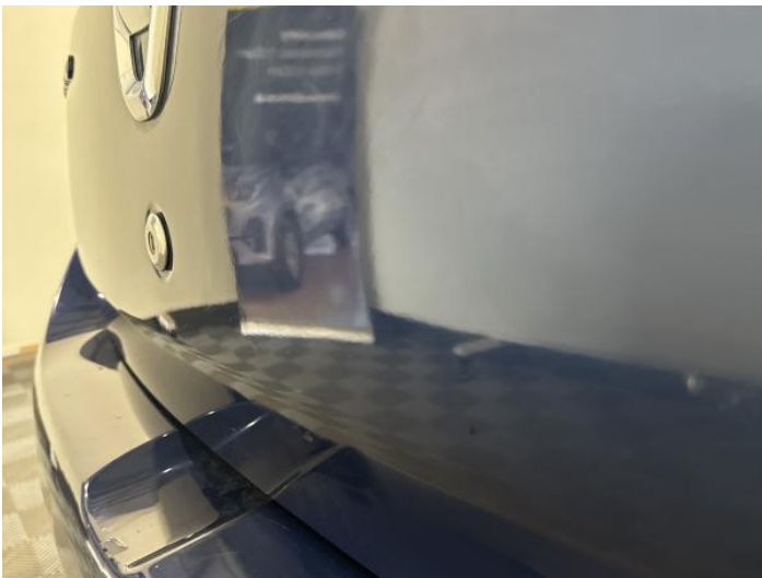
11: Tailgate Poor Previous Repair Rippled UpTo 30%
