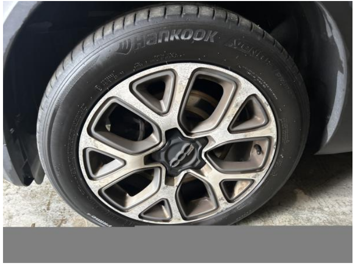
16: Wheel nsf Corroded Light
