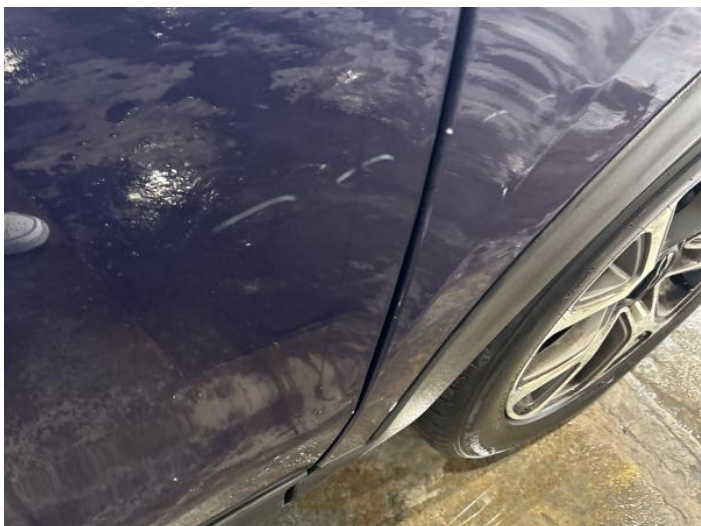
3: Door osf Scratched Over 25mm Thru Paint
