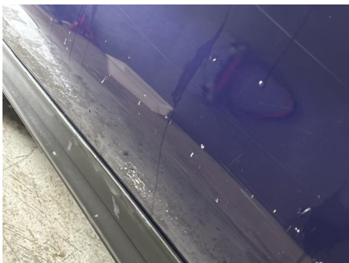
13: Door nsf Chipped Multiple Chips
