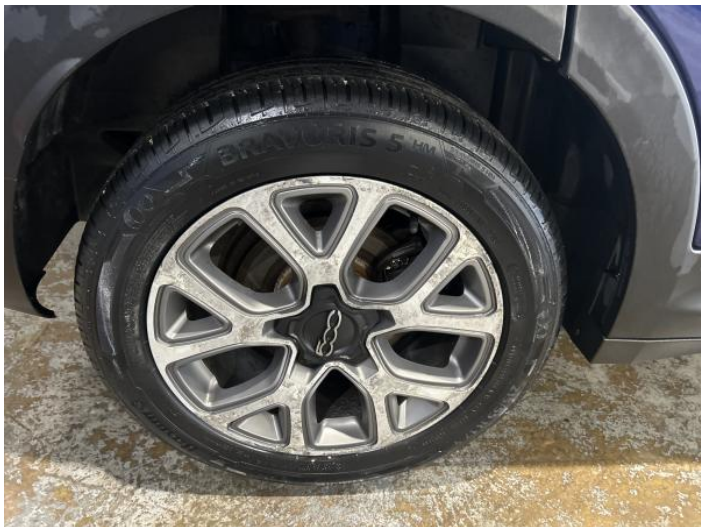
5: Wheel osr Corroded Light
