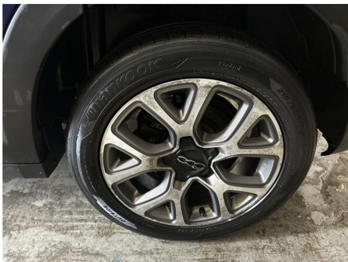
11: Wheel nsr Corroded Light
