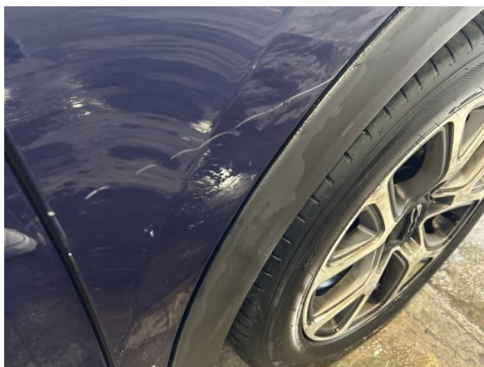
2: Wing osf Scratched Over 25mm Thru Paint
