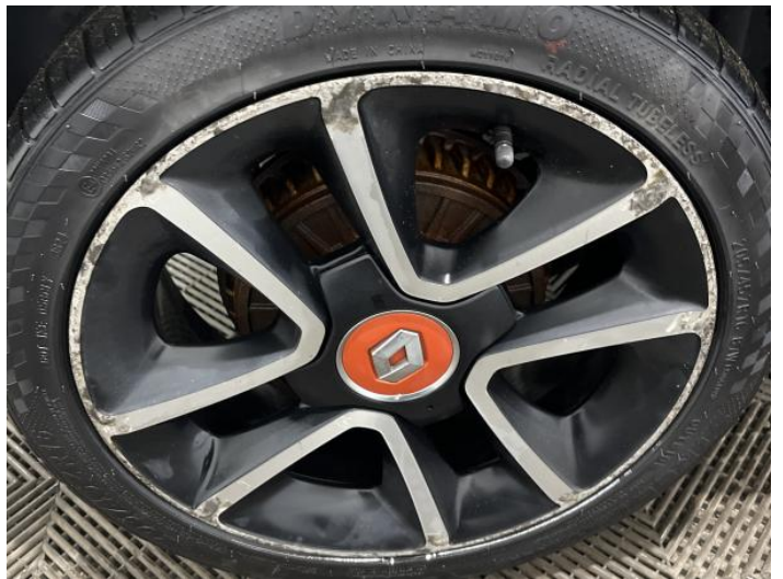
12: Wheel osr Scratched Over 50mm
