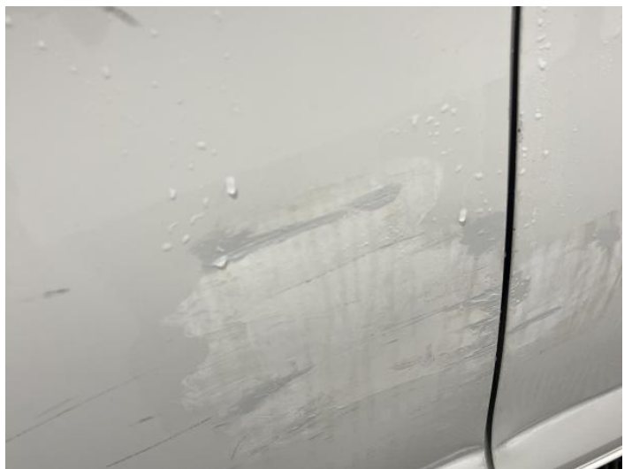
8: Qtr Panel osr Dented With Paint Damage
