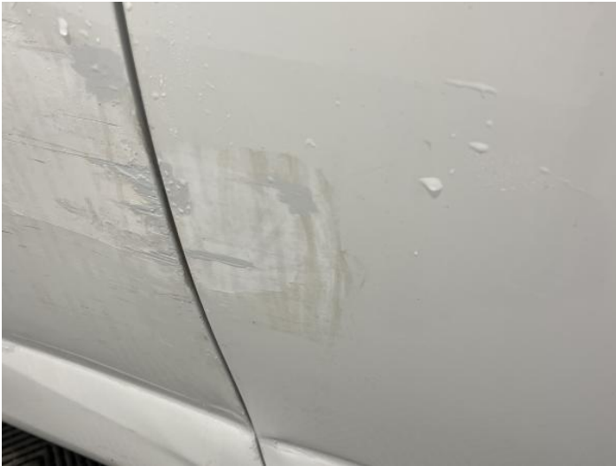
9: Door osf Dented With Paint Damage
