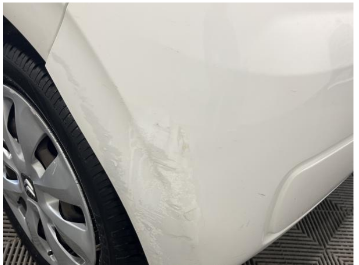
6: Bumper Rear Poor Previous Repair Poor Paint
