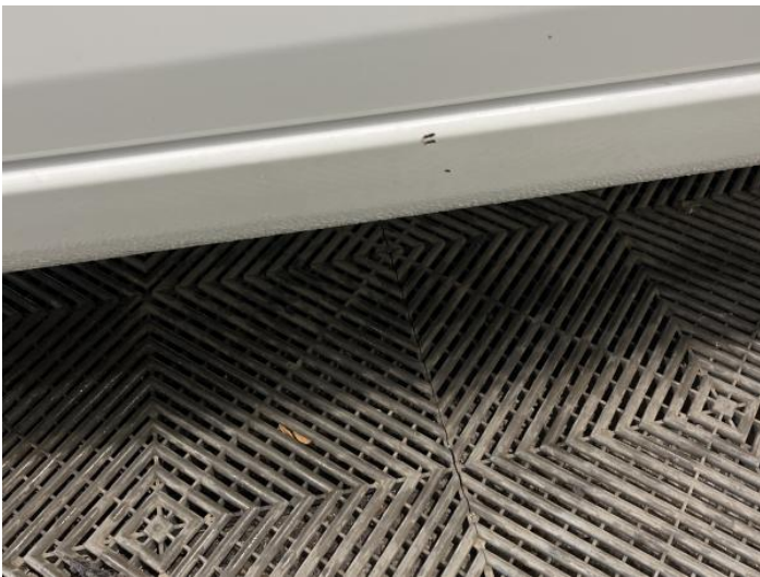
5: Sill ns Scratched Over 25mm Thru Paint
