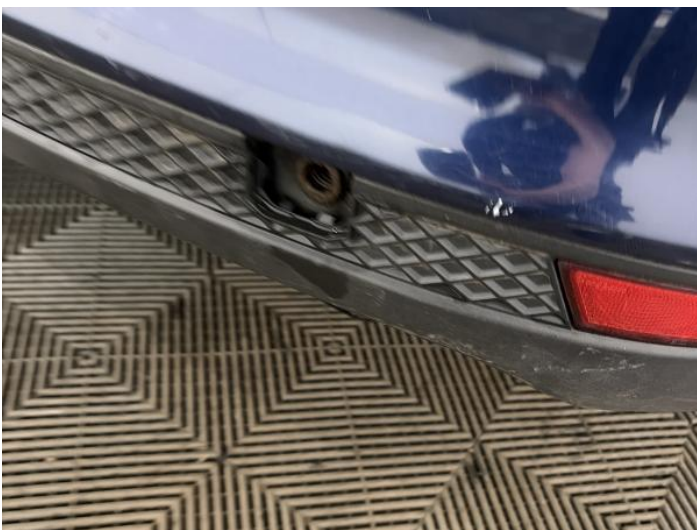
13: Rear TowEye Cvr Missing Replace
