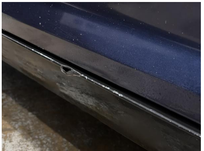
26: Sill Panel Trim os Broken Replace
