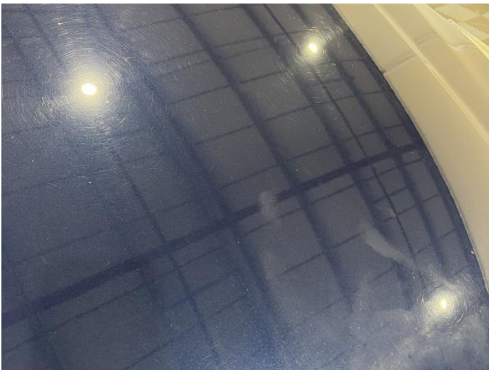
1: Bonnet Scratched Over 25mm Thru Paint
