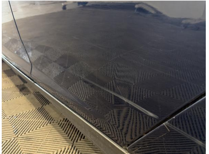
10: Door nsr Scratched Over 25mm Thru Paint
