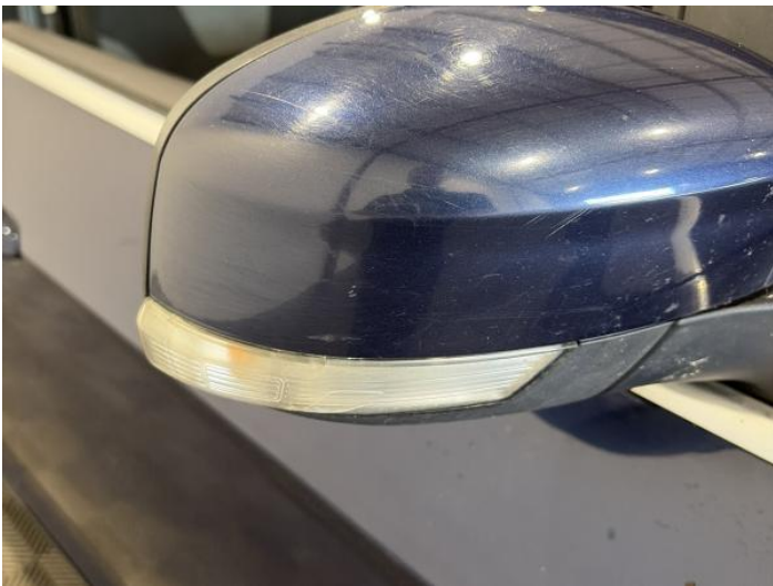
23: Flasher Side Repeater os Broken Replace
