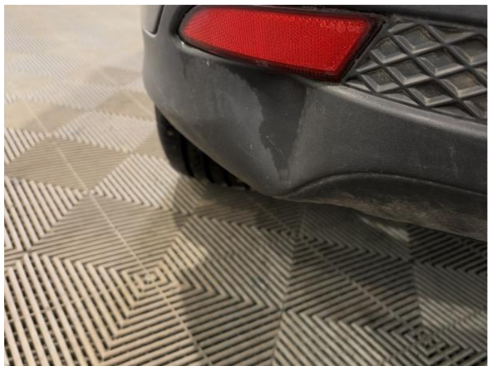
14: Bumper Rear Moulding Scuffed (Unpainted) Over 100mm
