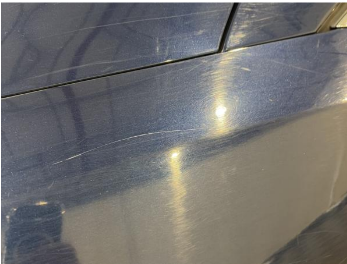
5: Wing nsf Scratched Over 25mm Thru Paint
