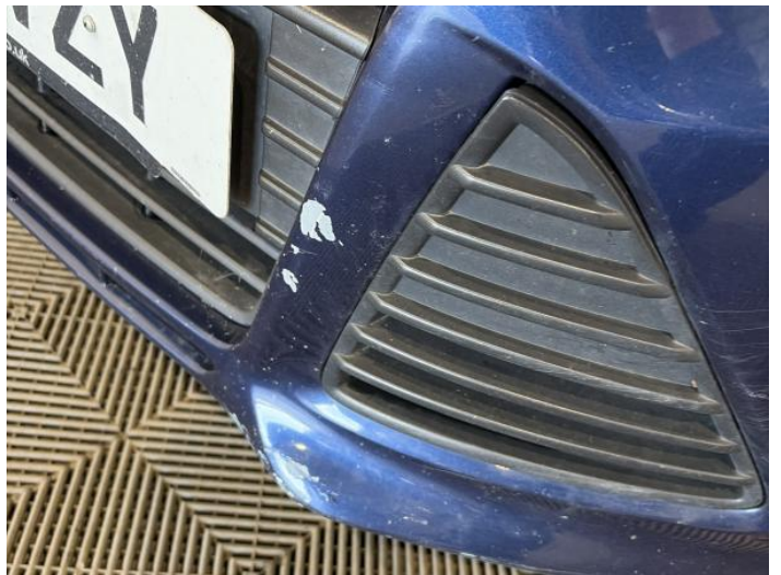
2: Bumper Front Dented With Paint Damage
