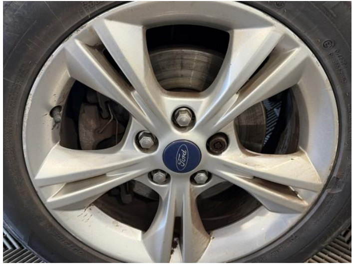
4: Wheel nsf Scratched Over 50mm
