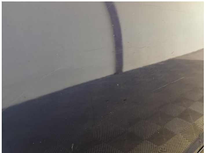
18: Door osr Scratched Over 25mm Thru Paint
