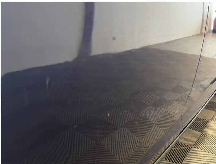
19: Door osr Dented Over 30mm
