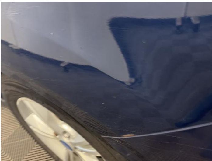
11: Qtr Panel nsr Scratched Rusted
