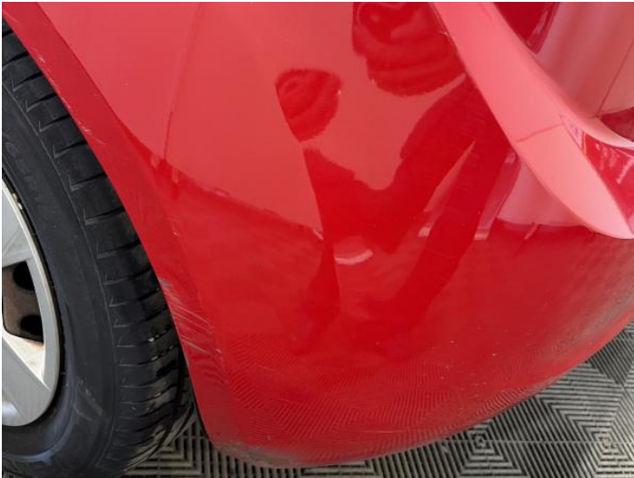
9: Bumper Rear Scratched 25 to 100mm Thru Paint
