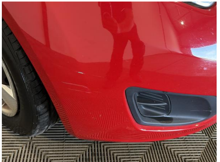
2: Bumper Front Scratched Over 100mm Thru Paint
