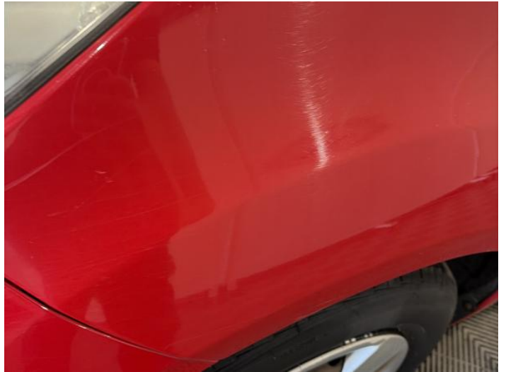
4: Wing nsf Scratched Over 25mm Thru Paint
