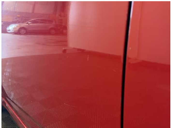
6: Door nsf Scratched Over 25mm Thru Paint
