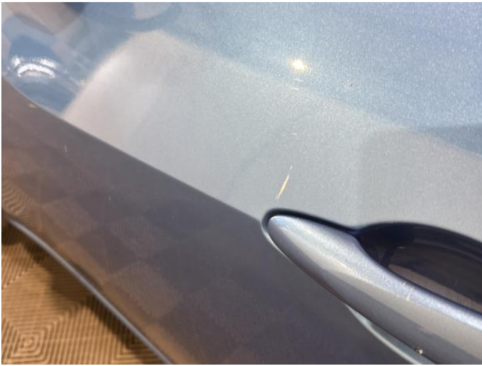
5: Door nsf Scratched Over 25mm Thru Paint
