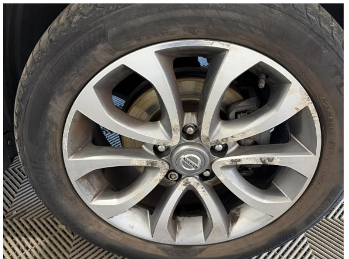
20: Wheel osf Scratched Over 50mm
