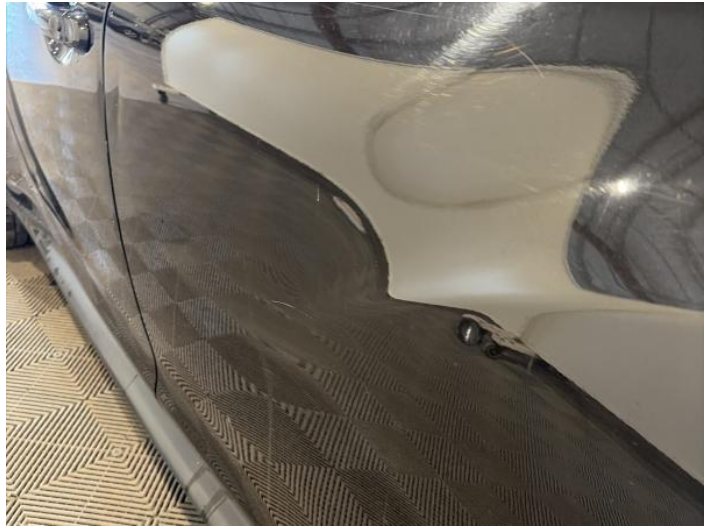
10: Door nsr Dented With Paint Damage
