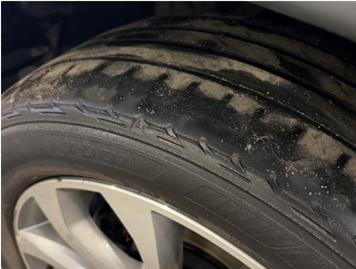
21: Tyre nsf Damaged Replace
