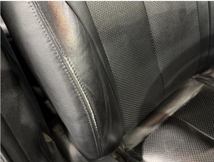
1: Seat Back Cover osf Scuffed Over 25mm
