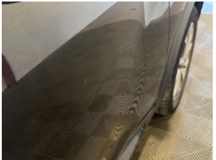
18: Door osf Dented Between 10mm + 30mm
