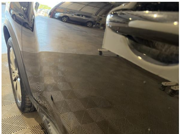
8: Door nsf Dented Between 10mm + 30mm
