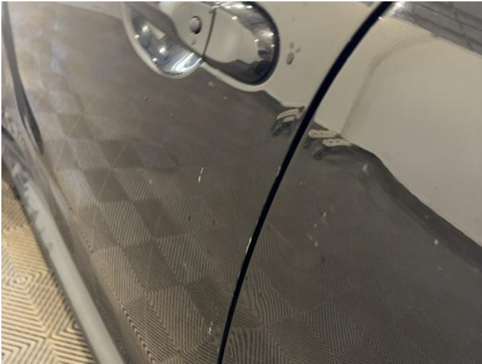
9: Door nsf Scratched Over 25mm Thru Paint
