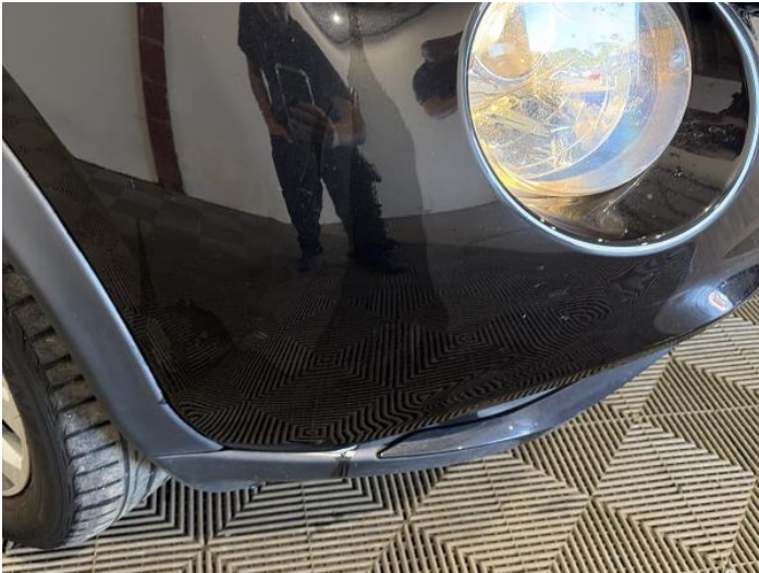
3: Bumper Front Scratched 25 to 100mm Thru Paint
