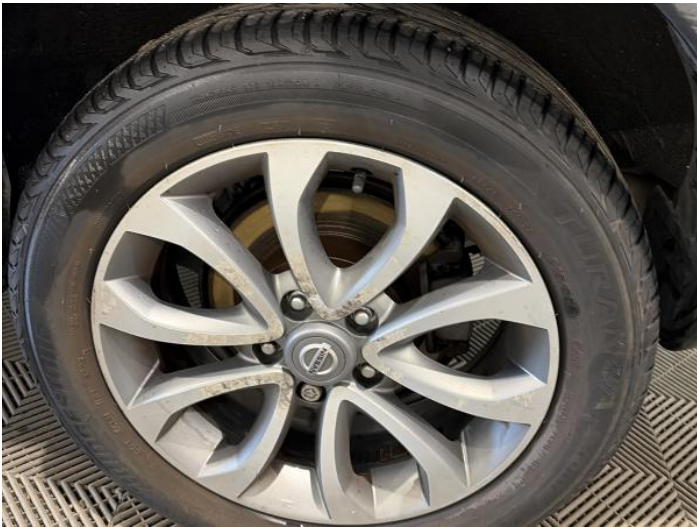
11: Wheel nsr Scratched Over 50mm
