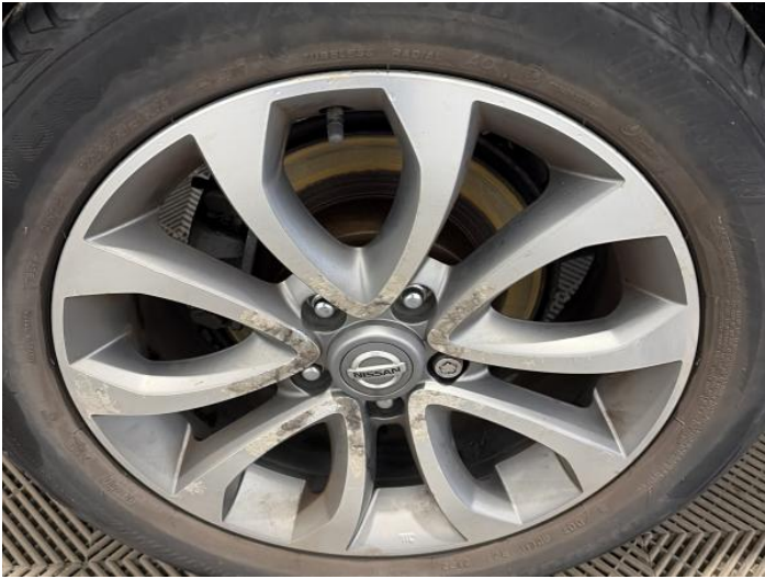
15: Wheel osf Scratched Over 50mm
