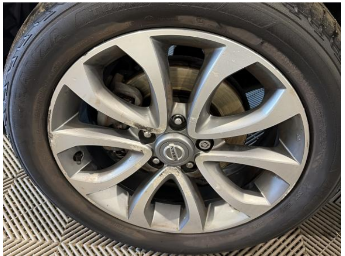
6: Wheel nsf Scratched Over 50mm
