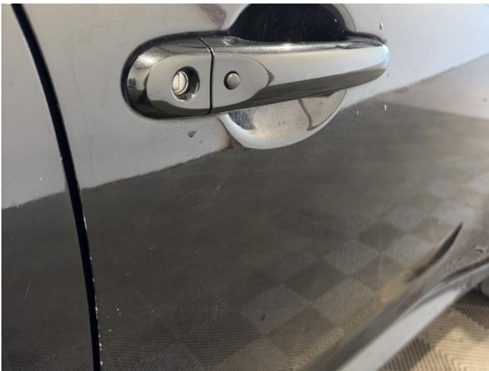
17: Door osf Chipped Edge Chip
