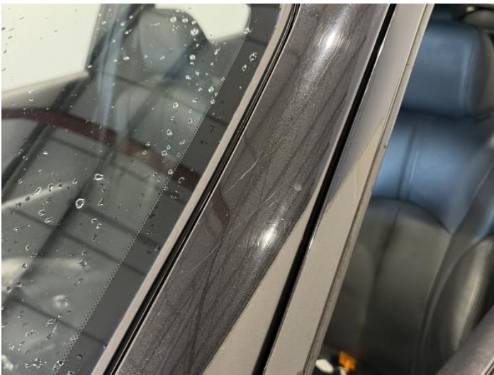
5: A Post ns Scratched UpTo 25mm Thru Paint
