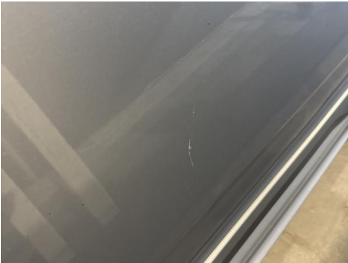
11: Door osf Scratched Over 25mm Thru Paint
