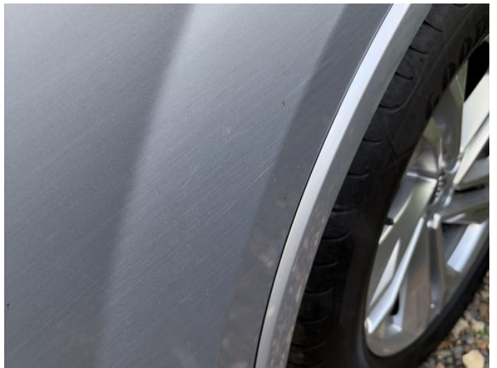
6: Door nsr Scratched Over 25mm Thru Paint
