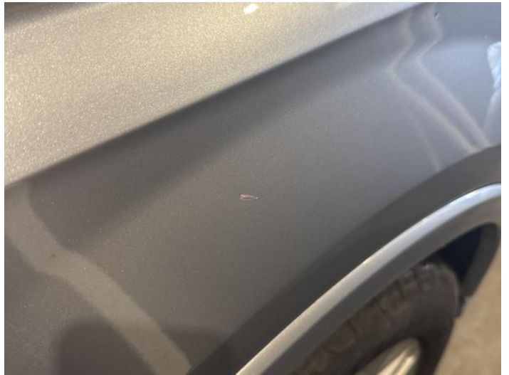
12: Wing osf Scratched UpTo 25mm Thru Paint
