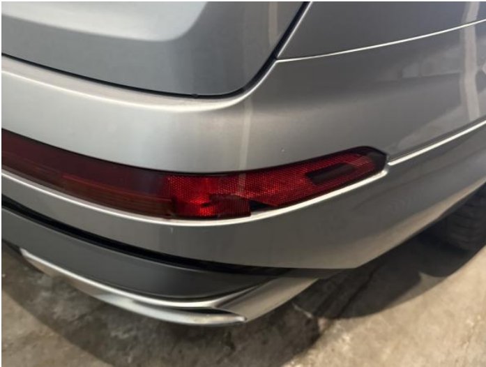
9: Bumper Reflector osr Broken Replace
