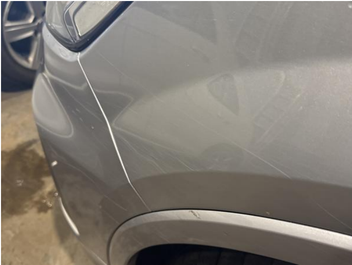
3: Wing nsf Scratched Over 25mm Thru Paint
