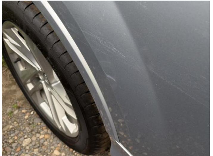
10: Door osr Dented With Paint Damage
