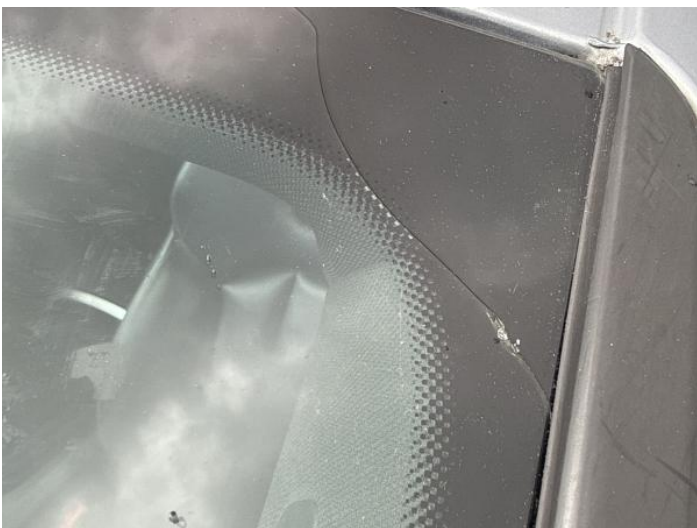
13: Screen Front Cracked Replace
