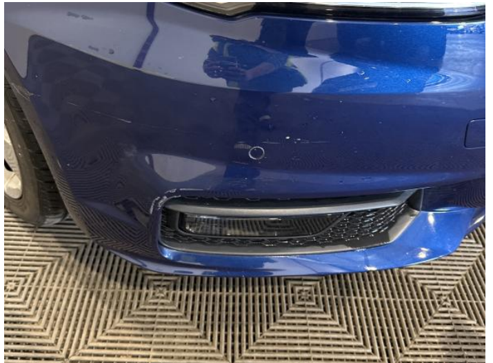
2: Bumper Front Scratched Over 100mm Thru Paint
