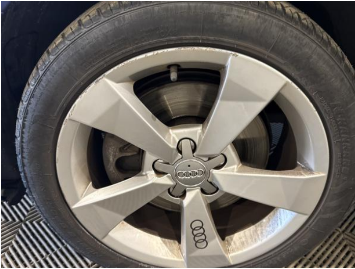
3: Wheel nsf Scratched Over 50mm
