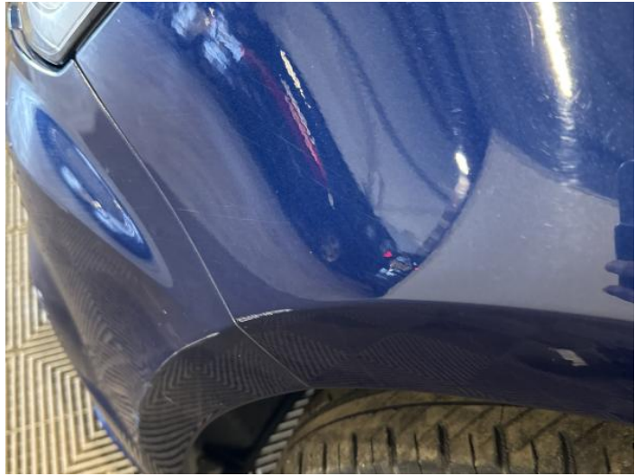
4: Wing nsf Scratched Over 25mm Thru Paint
