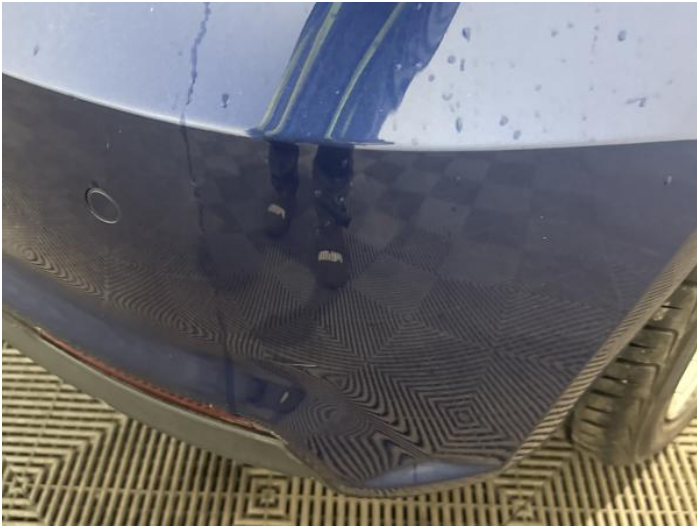
9: Bumper Rear Scratched Over 100mm Thru Paint
