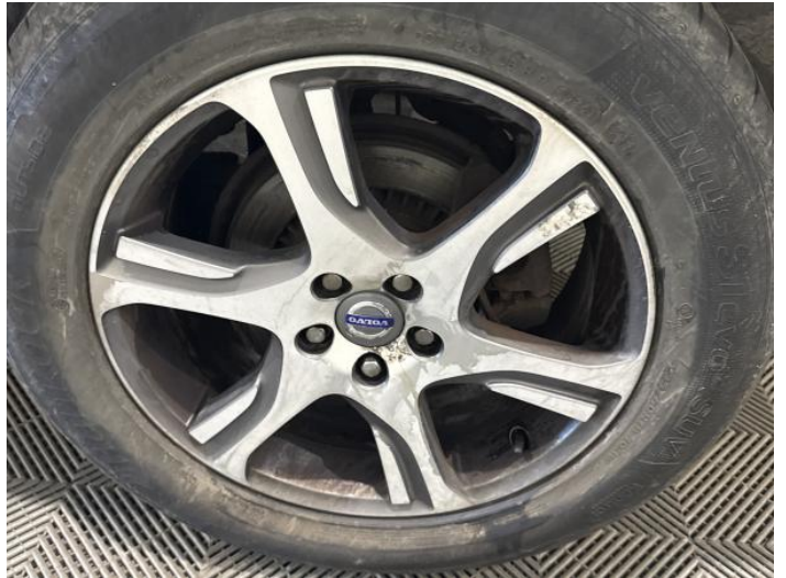
10: Wheel nsr Scratched Over 50mm
