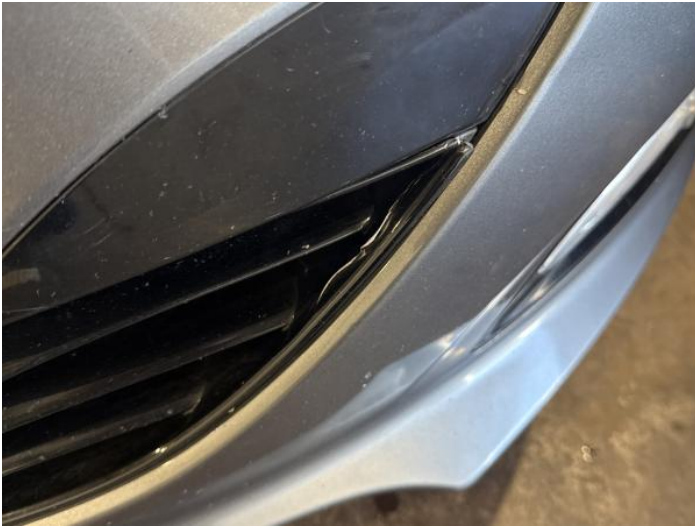
21: Bumper Front Grill Broken Replace
