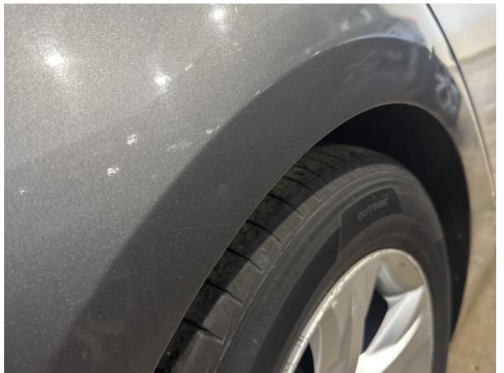
12: Qtr Panel osr Dented Between 10mm + 30mm
