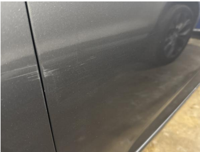
5: Door nsf Dented With Paint Damage
