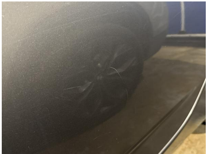
6: Door nsr Scratched Over 25mm Thru Paint
