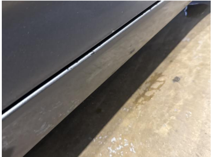
16: Sill Panel Trim ns Scratched (Painted) Over 25mm Thru Paint
