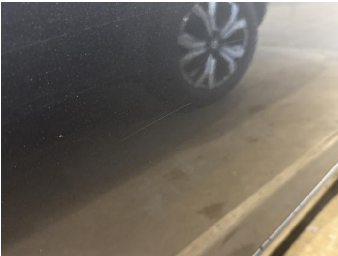
17: Door osf Scratched Over 25mm Thru Paint
