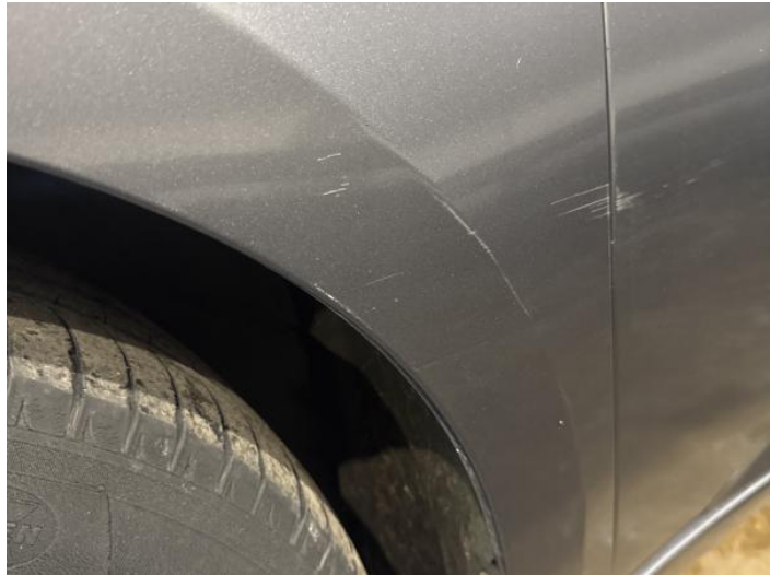
4: Wing nsf Scratched Over 25mm Thru Paint
