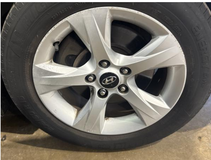
19: Wheel osf Scratched Over 50mm
