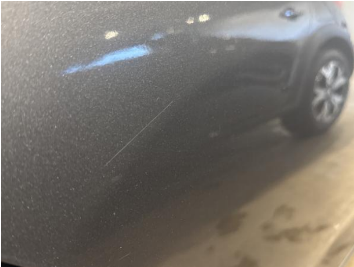
15: Door osr Scratched Over 25mm Thru Paint
