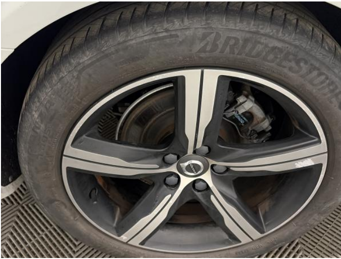
11: Wheel osr Scratched Over 50mm
