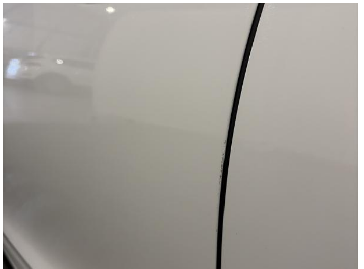
6: Door nsf Chipped Edge Chip
