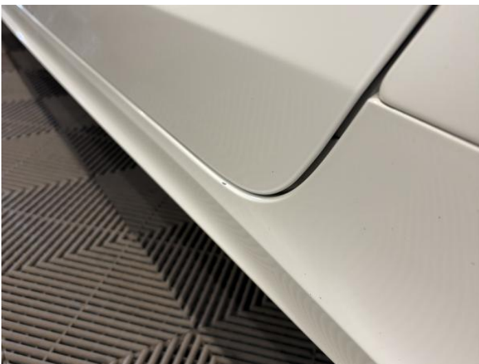
7: Sill ns Scratched UpTo 25mm Thru Paint
