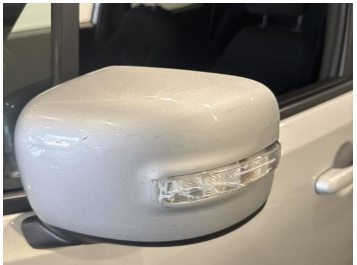
6: Flasher Side Repeater ns Broken Replace
