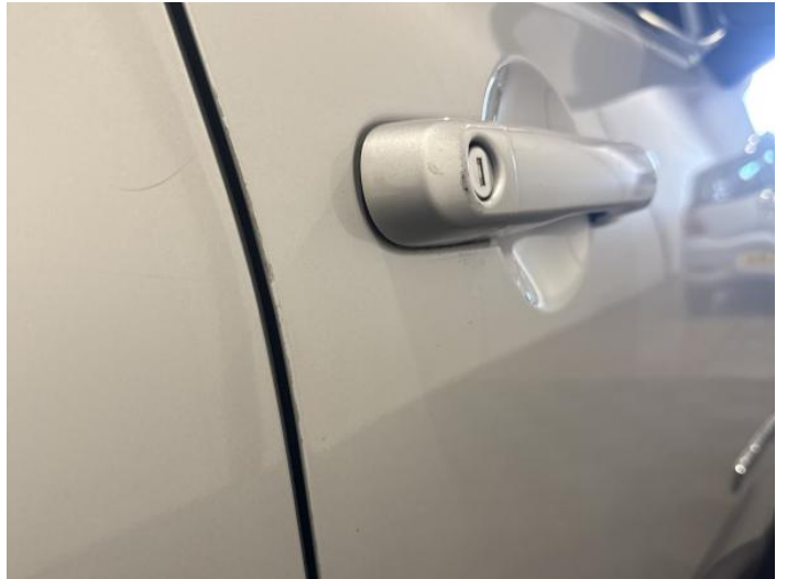
16: Door osf Chipped Edge Chip
