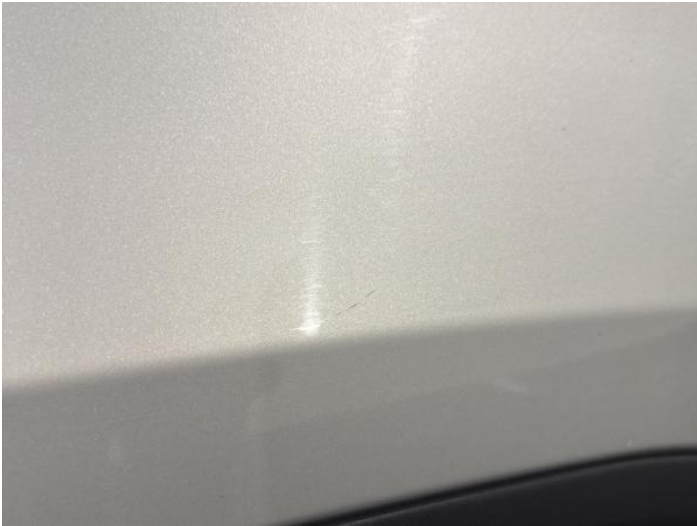
3: Wing nsf Scratched UpTo 25mm Thru Paint
