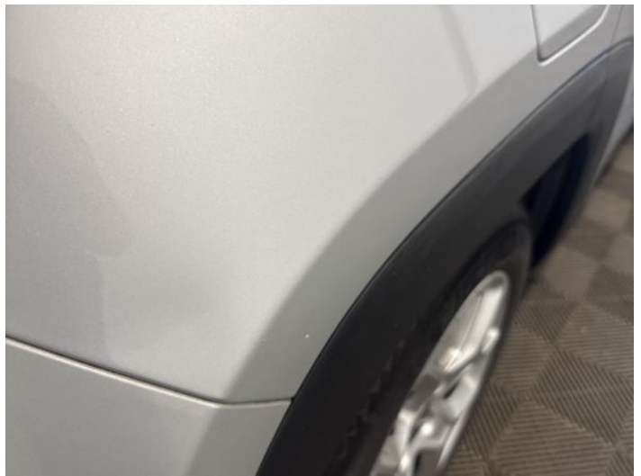
12: Qtr Panel osr Dented Over 30mm
