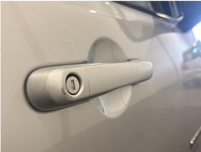
17: Handle Outer osf Scratched (Painted) UpTo 25mm Thru Paint
