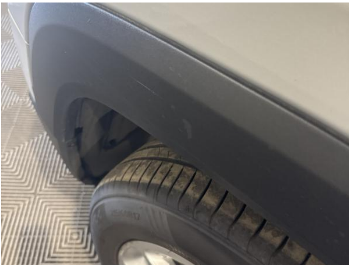
5: Wing Front Arch Extension ns Scuffed (Unpainted) Over 100mm
