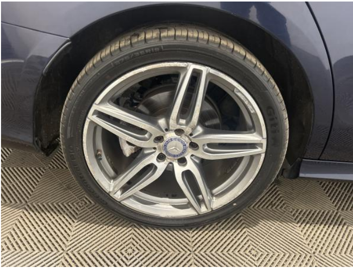
5: Wheel osr Corroded Light
