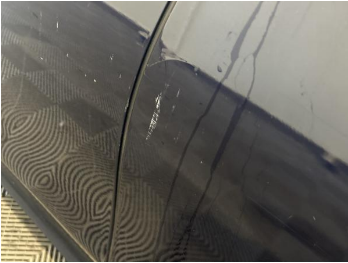
9: Door nsr Scratched Over 25mm Thru Paint
