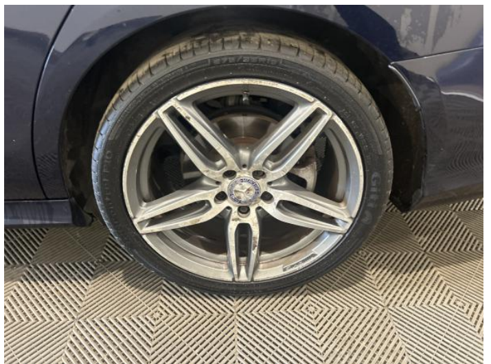
8: Wheel nsr Corroded Light
