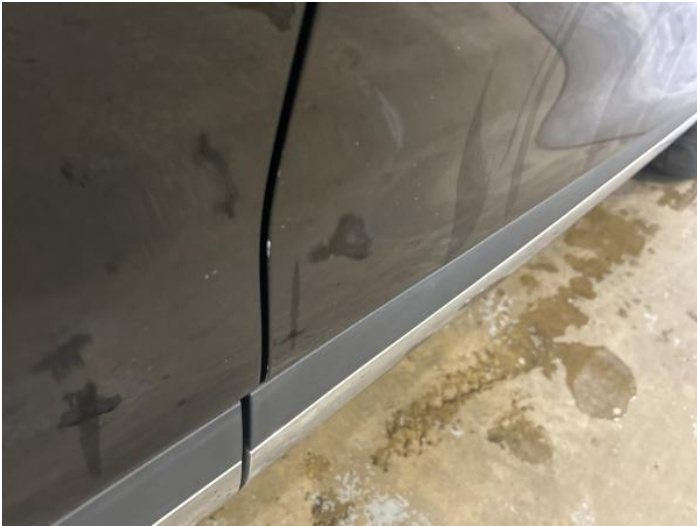
3: Door osf Chipped Edge Chip
