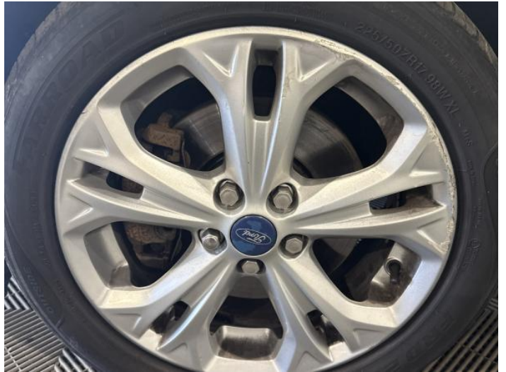
4: Wheel nsf Scratched Over 50mm
