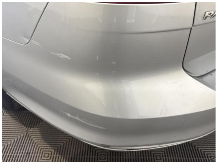
8: Bumper Rear Scratched 25 to 100mm Thru Paint
