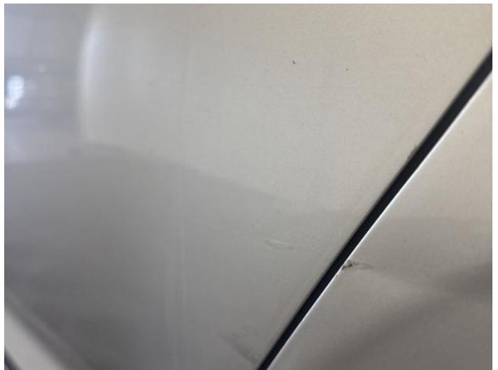
6: Door nsr Scratched Over 25mm Thru Paint
