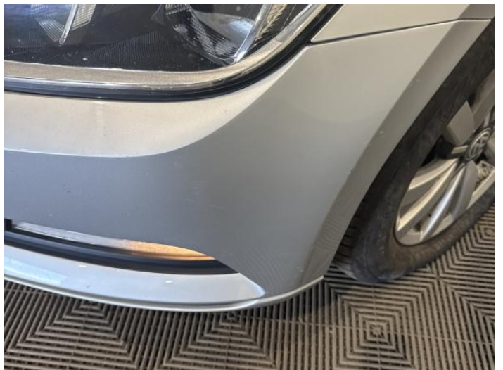
2: Bumper Front Scratched 25 to 100mm Thru Paint
