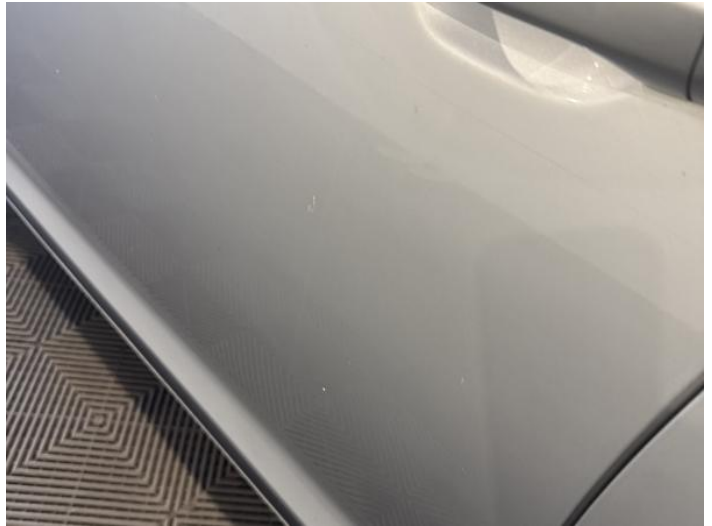
4: Door nsf Scratched Over 25mm Thru Paint
