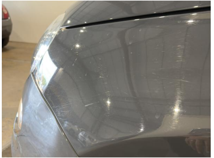
4: Wing nsf Scratched UpTo 25mm Thru Paint
