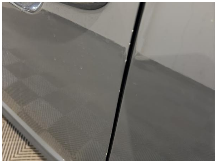
8: Door nsf Chipped Edge Chip
