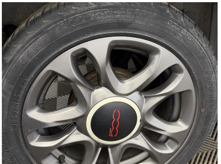
14: Wheel osr Scratched Over 50mm
