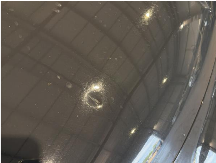
1: Bonnet Dented With Paint Damage
