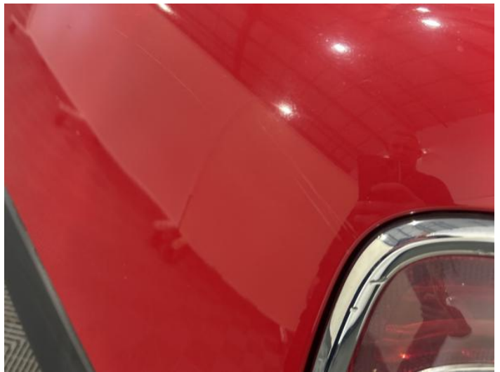
6: Qtr Panel nsr Scratched Over 25mm Not Thru Paint
