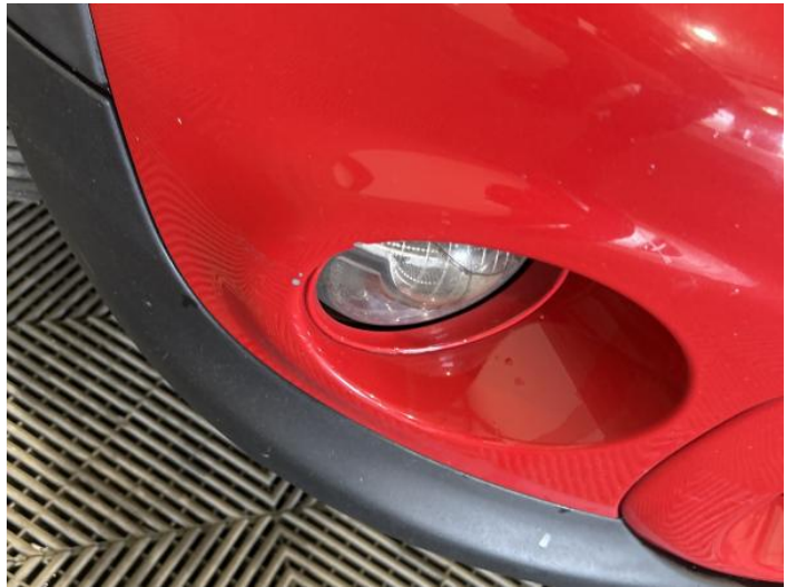
12: Bumper Front Chipped Multiple Chips
