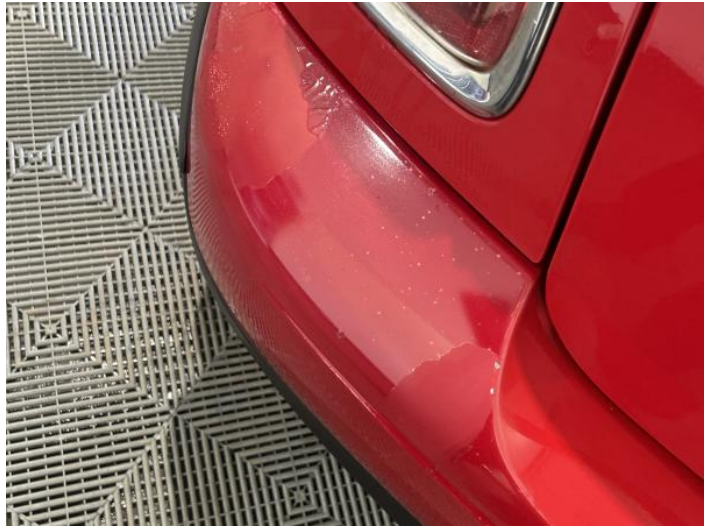
4: Bumper Rear Poor Previous Repair Paint Flake
