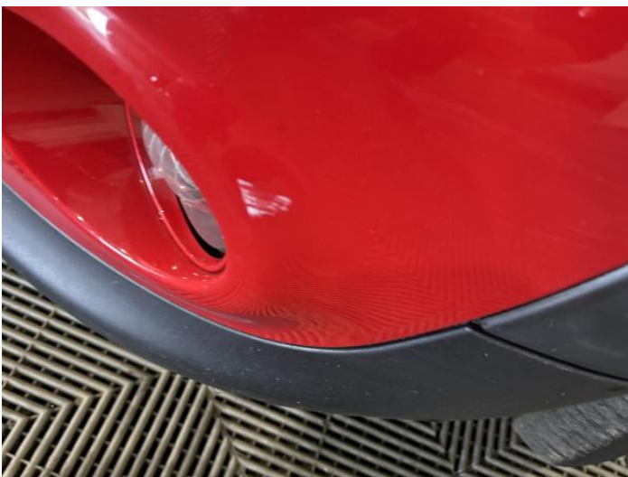
13: Bumper Front Scratched UpTo 25mm Thru Paint
