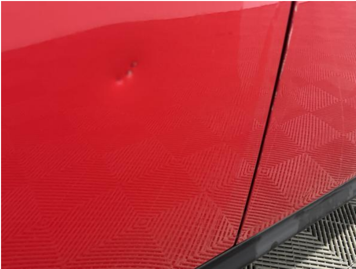
3: Qtr Panel osr Dented With Paint Damage
