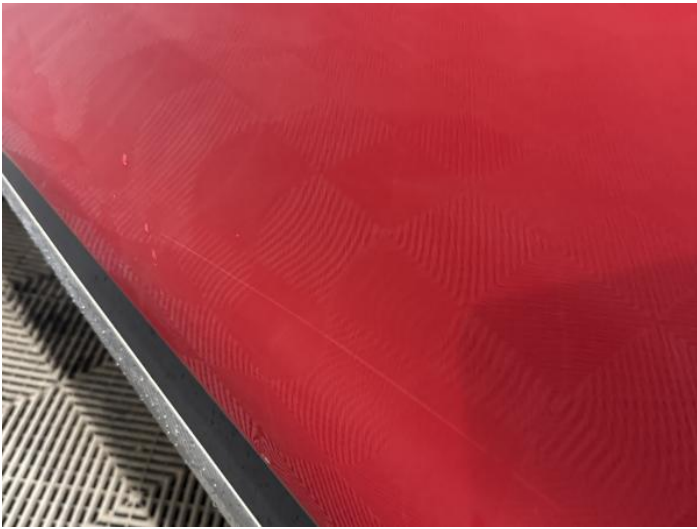
5: Door nsf Scratched Over 25mm Thru Paint
