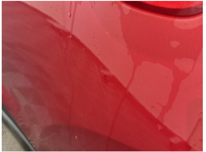
6: Door nsr Scratched Over 25mm Thru Paint
