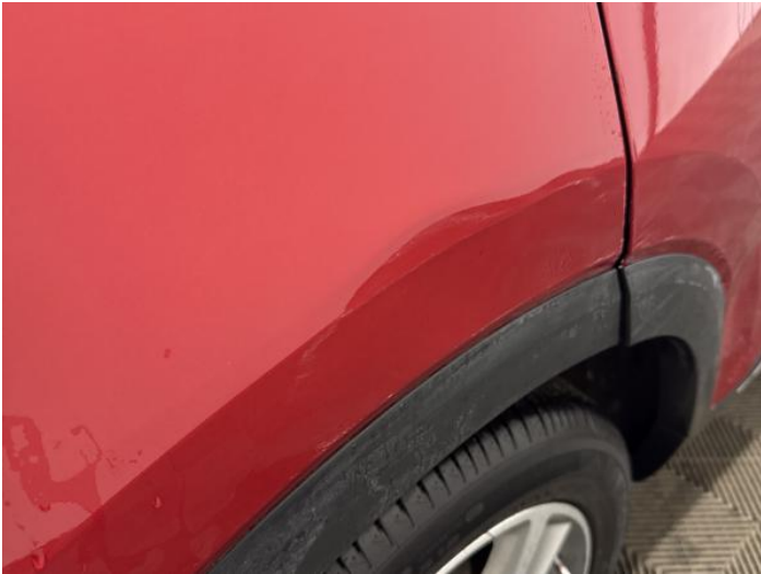
9: Qtr Panel osr Dented With Paint Damage
