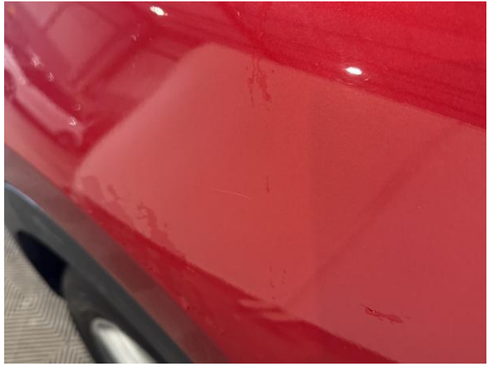
4: Wing nsf Scratched Over 25mm Thru Paint
