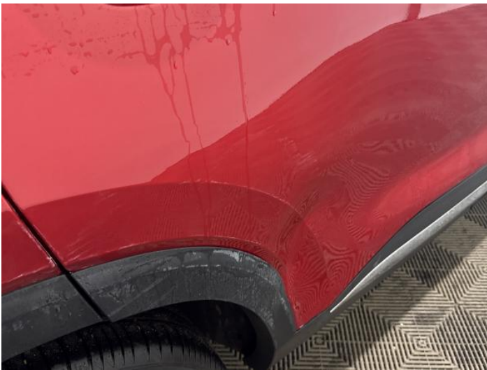
11: Door osr Dented With Paint Damage
