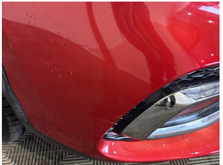
2: Bumper Front Scratched 25 to 100mm Thru Paint
