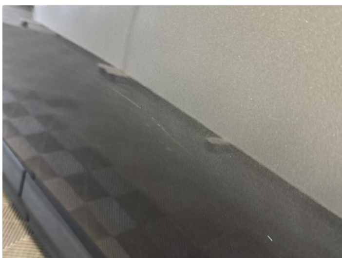
7: Door nsr Scratched Over 25mm Thru Paint
