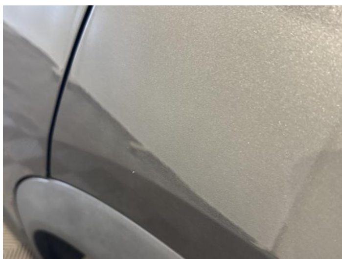
8: Qtr Panel nsr Chipped 1 To 5
