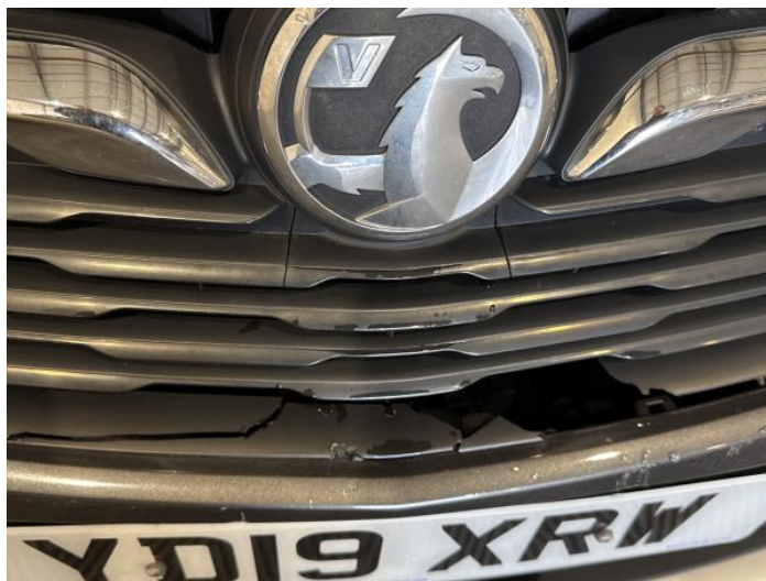
2: Bumper Front Grill Broken Replace
