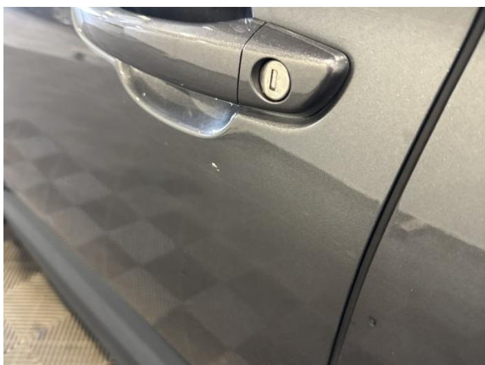
5: Door nsf Dented Between 10mm + 30mm
