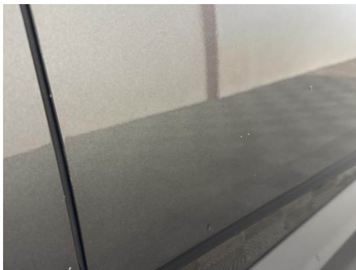
12: Door osf Dented Between 10mm + 30mm
