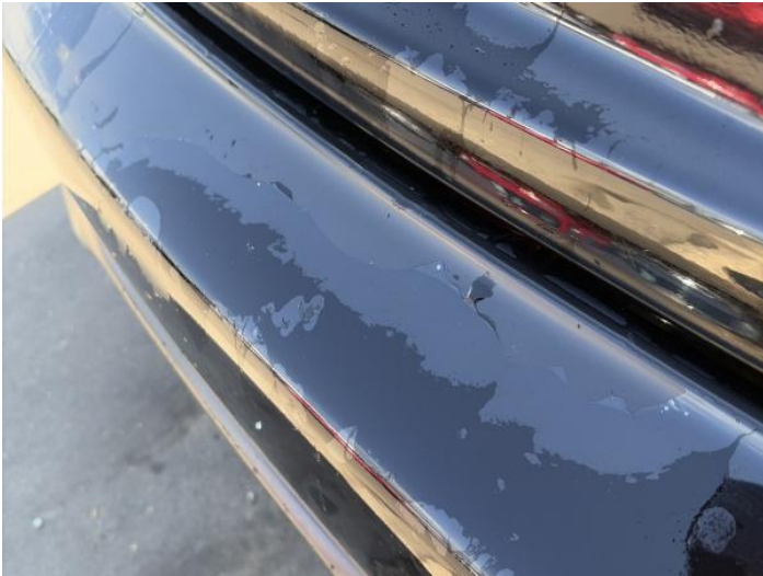
9: Bumper Rear Poor Previous Repair Paint Flake
