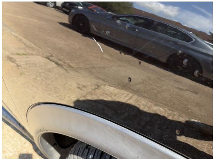
2: Wing of Scratched Up To 25mm Thru Paint
