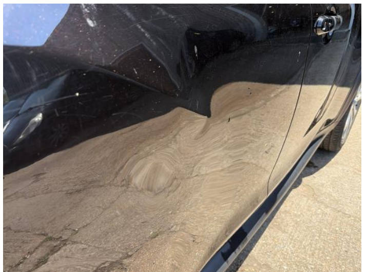
8: Door osr Dented Over 30mm
