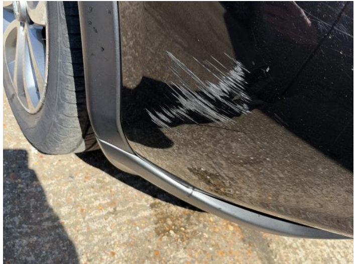
10: Bumper Front Scratched Over 100mm Thru Paint
