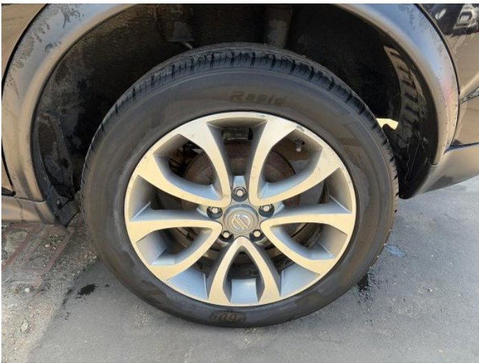
5: Wheel osf Corroded Light
