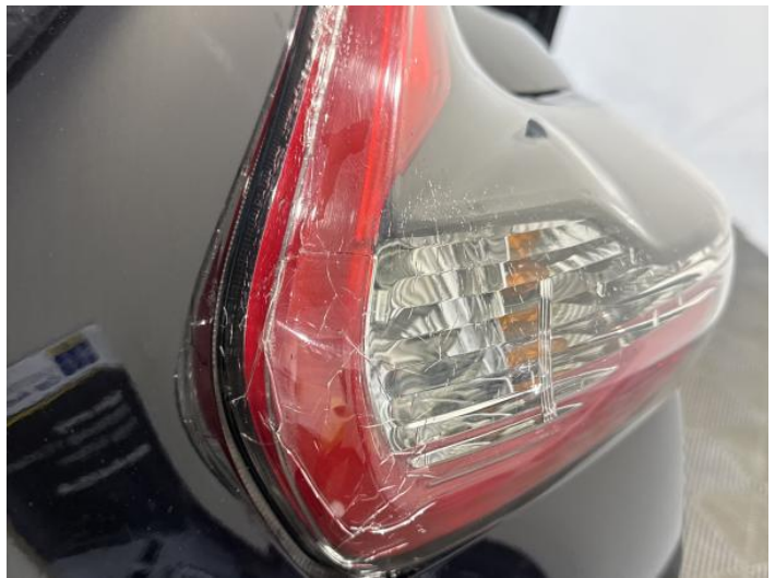
18: Lamp osr Broken Replace
