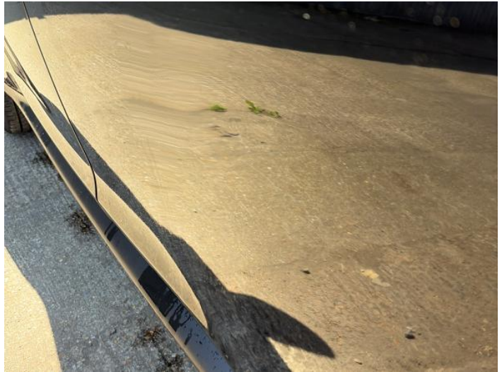
16: Door nsr Dented 2 Or Less UpTo 10mm
