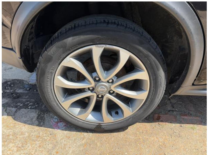
6: Wheel osr Corroded Light
