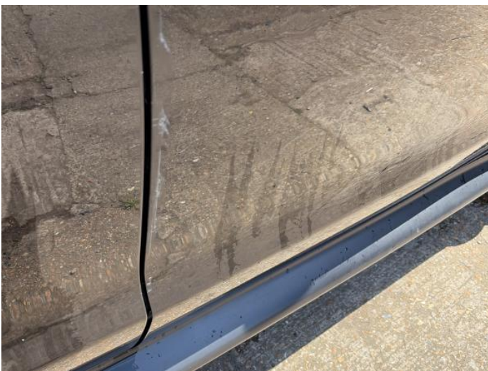
7: Door osf Dented With Paint Damage
