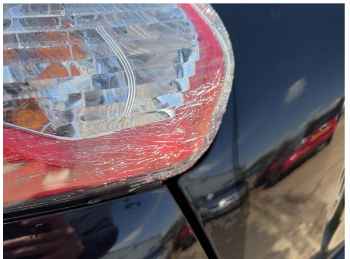
14: Lamp nsr Broken Replace
