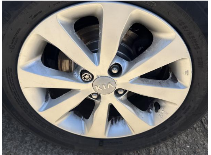
10: Wheel nsr Scratched Over 50mm
