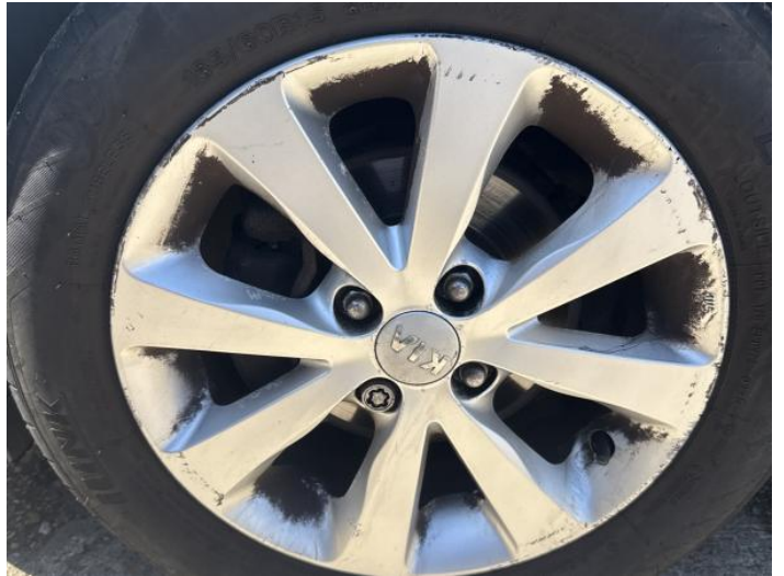
4: Wheel nsf Scratched Over 50mm
