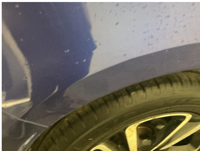
16: Qtr Panel osr Poor Previous Repair Paint Flake
