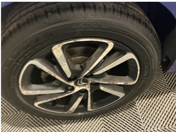
15: Wheel osr Scratched Over 50mm
