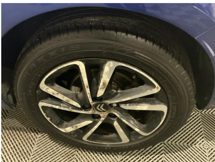
11: Wheel nsr Scratched Over 50mm
