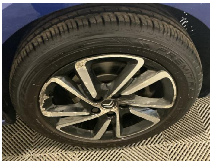
20: Wheel osf Scratched Over 50mm
