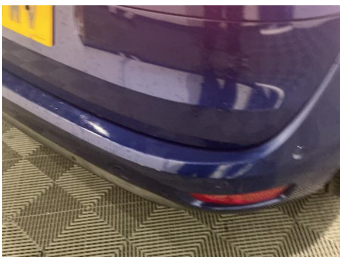
13: Bumper Rear Scratched Over 100mm Thru Paint
