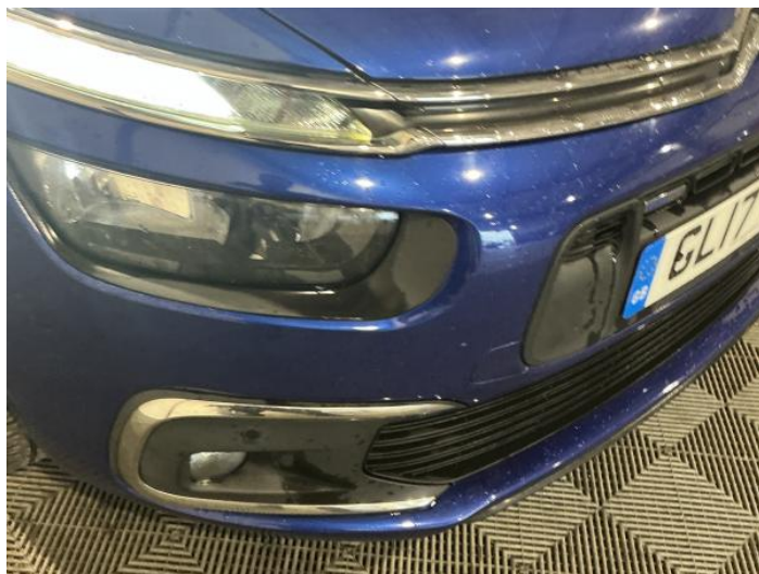
2: Bumper Front Chipped Multiple Chips
